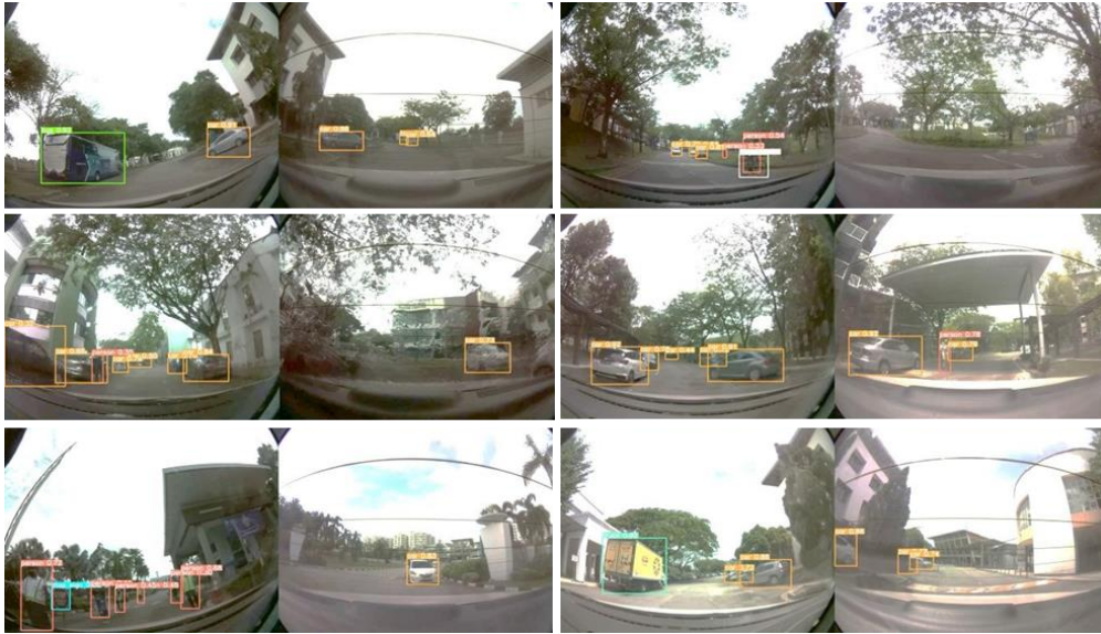
Figure 17. Examples of scenarios captured by the instrumented vehicle focusing on parked vehicles, cyclist and pedestrians along the road
