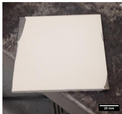
Figure 1. Sample with applied layer of flux powder
