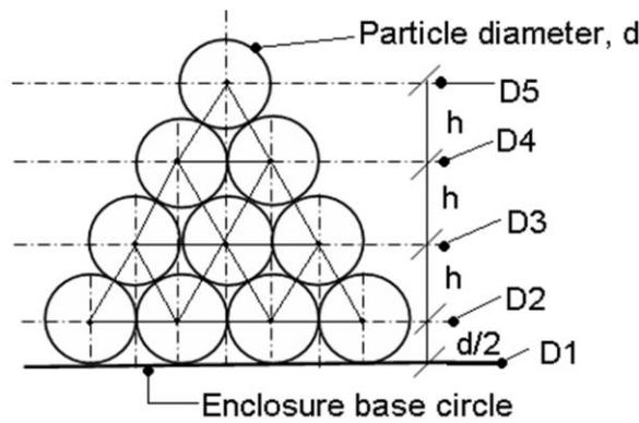
Figure 4. Particle arrangement in enclosure with simplified geometry
