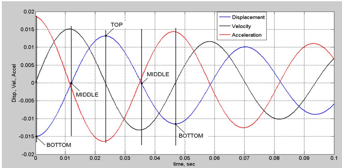
Figure 6. Displacement, velocity, and acceleration curves under transient excitation
