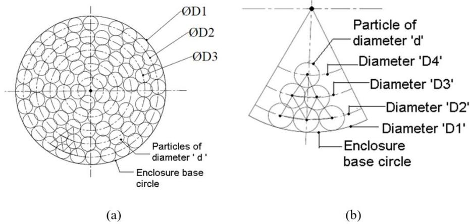
Figure 3. Arrangement of particles in enclosure: (a) In one layer and (b) Small sector of particle arrangement
