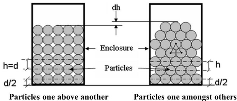
Figure 5. Particle arrangement in different layers in the enclosure
