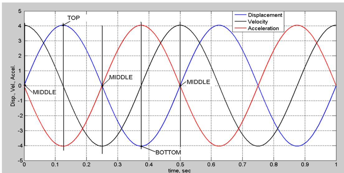
Figure 7. Displacement, velocity, and acceleration curves under forced excitation
