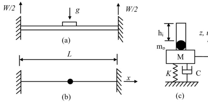
Figure 2. Theoretical modeling of fixed-fixed beam with PID: (a) A schematic of the fixed-fixed beam and enclosure, (b) A model of fixed-fixed beam with end mass and (c) The equivalent single degree of freedom system
