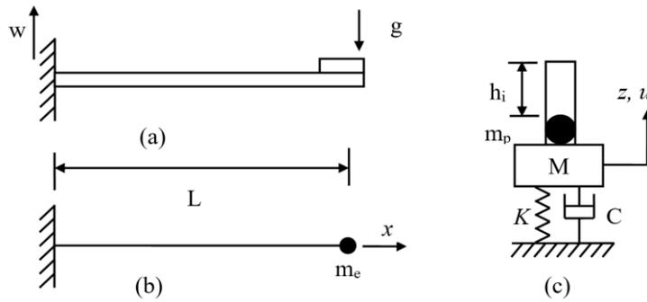
Figure 1. Theoretical modeling of cantilever beam with PID: (a) A schematic diagram of cantilever beam and enclosure, (b) A model of the beam with end mass, and (c) The equivalent single degree of freedom system
