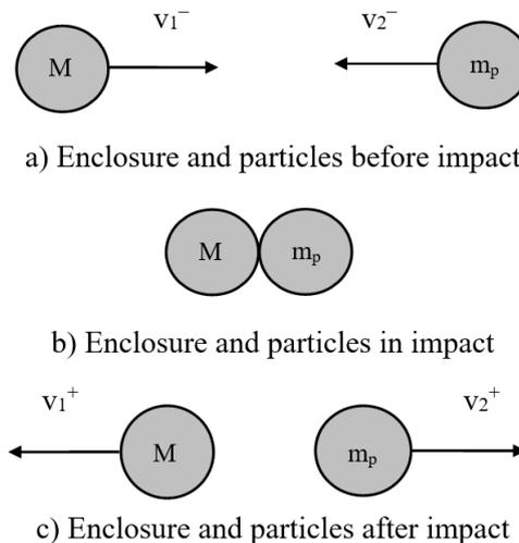
Figure 8. Collision mechanism of enclosure mass and particle mass: (a) before impact, (b) during impact and (c) after impact
