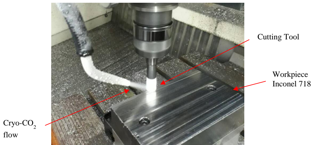
Figure 1. High-speed milling process under cryogenic CO 2 condition
