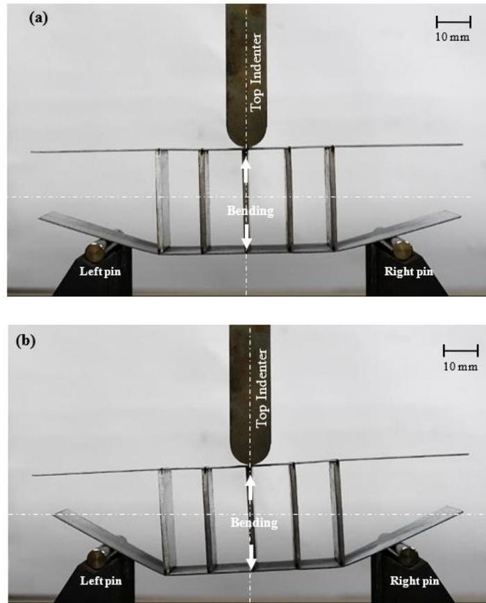
**Figure 7.** (a) and (b) Photographs of damage development in five cores with spacing distance,  $s = 19$  mm
