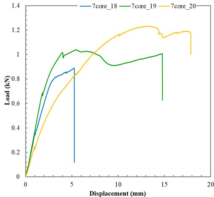
**Figure 14.** Load-displacement trace on three-point bending test of seven cores with different spacing distances,  $s = 18$ , 19, and 20 mm
