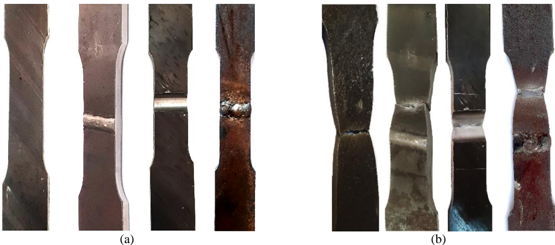
Figure 4. Experimental set up: (a) Before failure and (b) After failure
