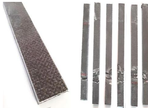
Figure 4. Tensile test specimens before and after fracture
