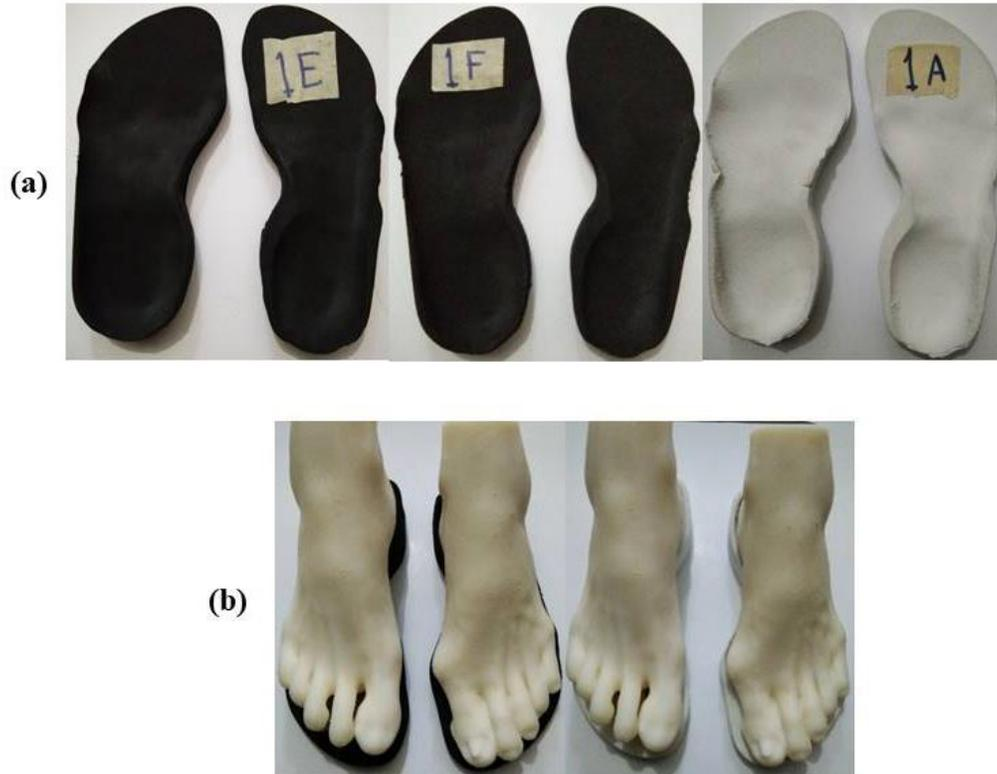
Figure 3. Research output: (a) Product insoles of EVA foam with different hardness, (b) confirmation insole product with 3D prototype foot of patient with diabetic.
