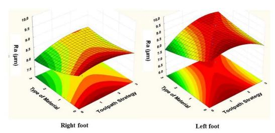
Figure 5. (c) Plot 3D curve of Ra vs Type of Material Eva Rubber foam – Toolpath Strategy
