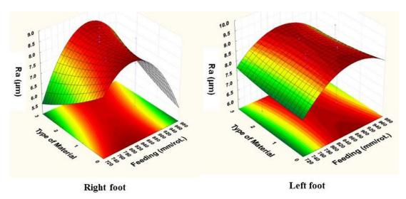
Figure 5. (a) Plot 3D curve of Ra vs Type of Material Eva Rubber foam – Feeding (mm/min).
