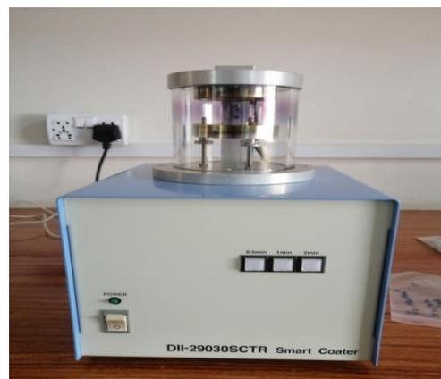
**Figure 8.** Specimen surface coater machine
