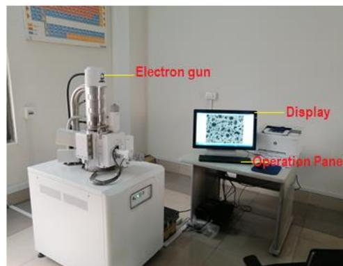
**Figure 7.** Scanning electron microscope setup
