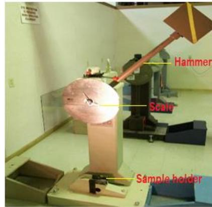
**Figure 6.** Charpy impact test machine
