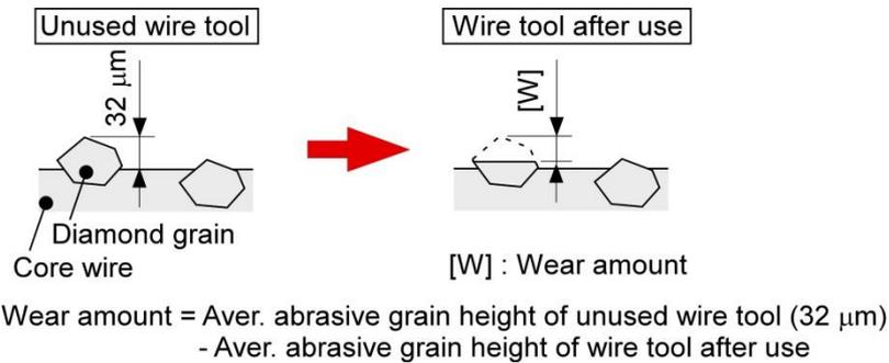
**Figure 4.** Definition of the amount of wear of the electroplated diamond wire tool in this study
