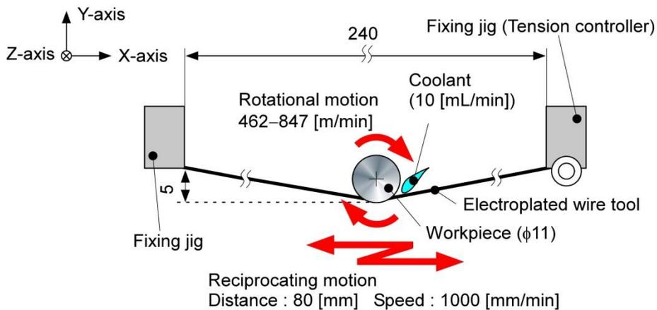
**Figure 2.** Schematic diagram of the machining process viewed from the Z-axis direction
