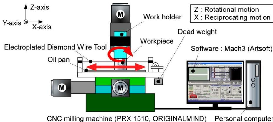
**Figure 1.** Schematic diagram of the experimental setup, which is a modified tabletop CNC milling machine
