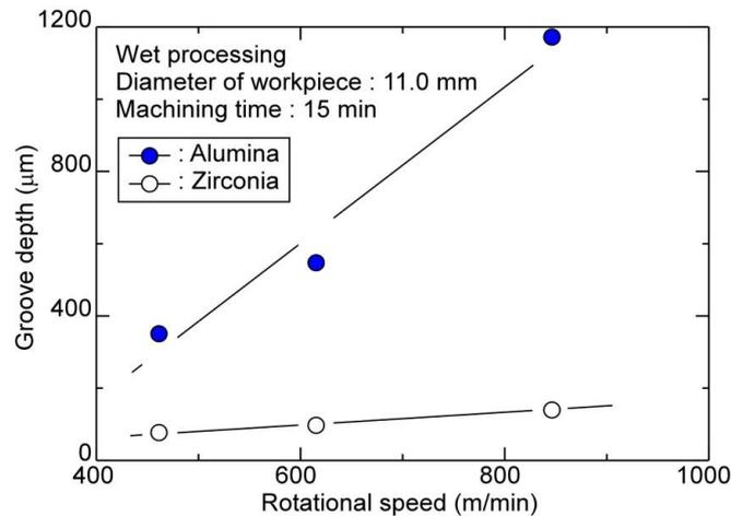
**Figure 8.** Relationship between the rotational speed of the workpiece and the groove depth
