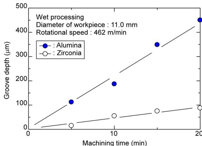
**Figure 5.** Relationship between machining time and groove depth
