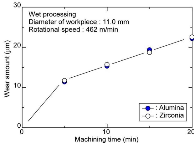
**Figure 6.** Relationship between machining time and the wear of the electroplated diamond wire tool
