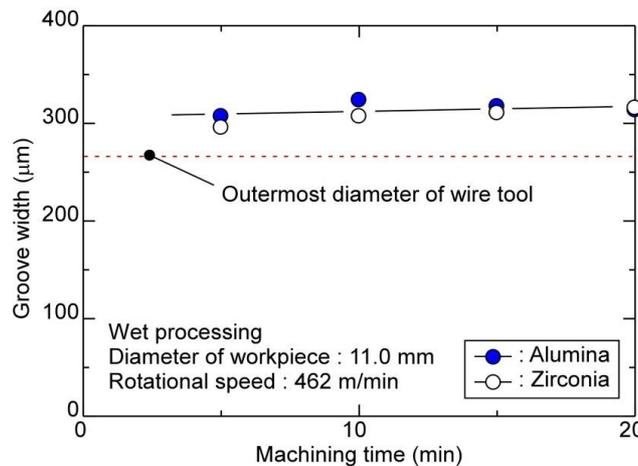
**Figure 7.** Relationship between machining time and the groove width
