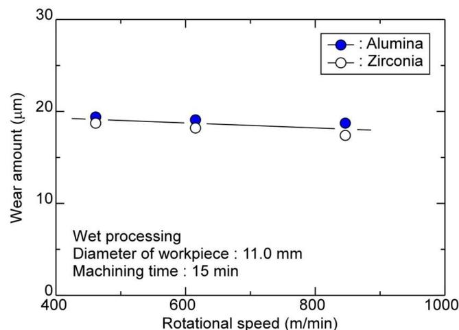
**Figure 9.** Relationship between the rotational speed of the workpiece and the wear of the wire tool
