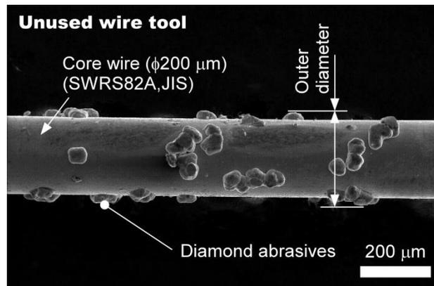
**Figure 3.** Appearance of an unused electroplated diamond wire tool
