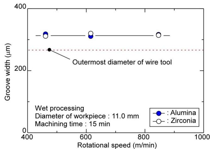
**Figure 10.** Relationship between the rotational speed of the workpiece and the groove width
