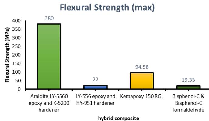
**Figure 8.** Flexural properties of carbon-jute FRPC fabricated using hand lay-up technique
