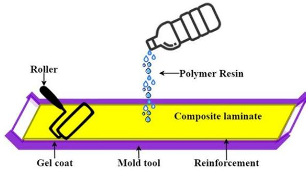
Figure 1. Block diagram of a basic hand layup method
