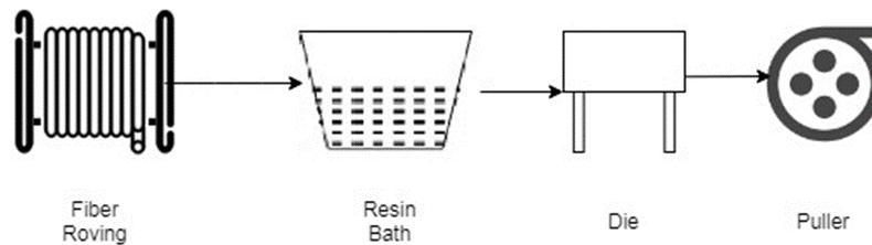
**Figure 5.** Pultrusion process [28]
