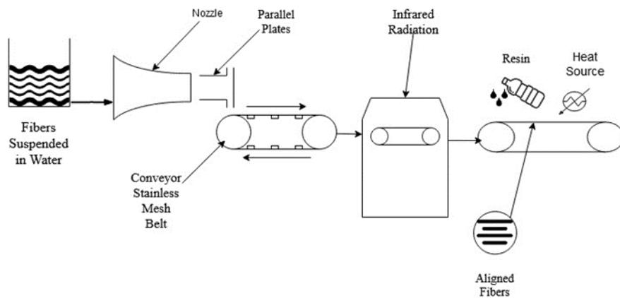
**Figure 3.** Block diagram of HiPerDiF process
