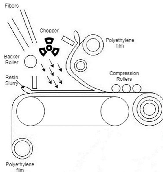
**Figure 6.** Sheet molding compound [30]
