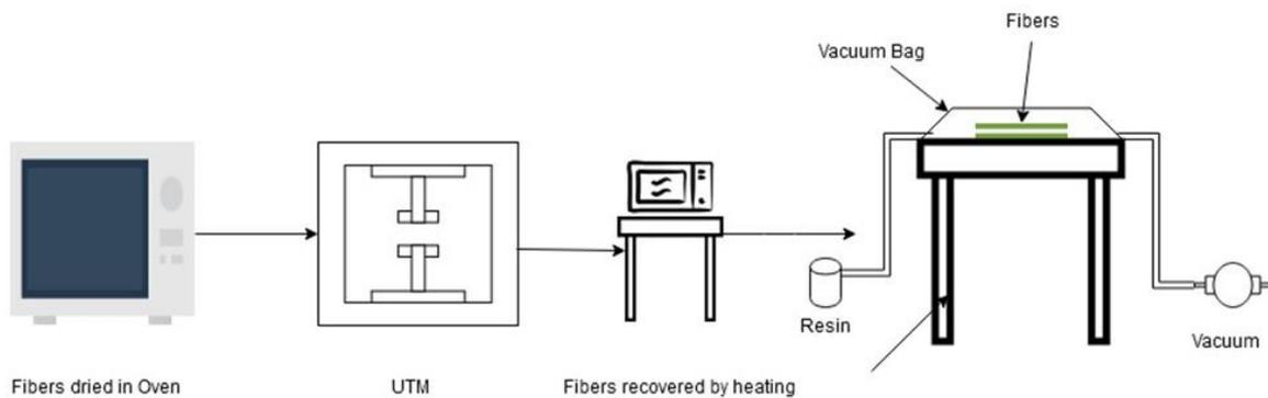
**Figure 4.** Block diagram of VARI process [27]
