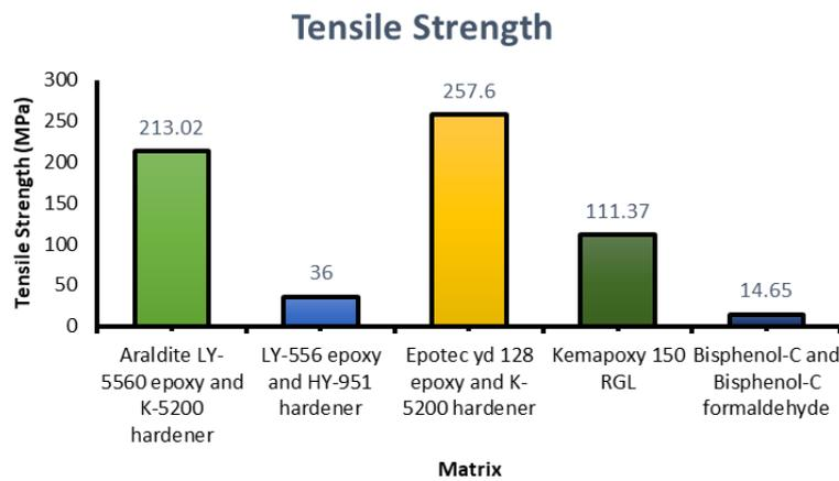
**Figure 7.** Tensile properties of carbon-jute epoxy hybrid composites fabricated using hand lay-up technique
