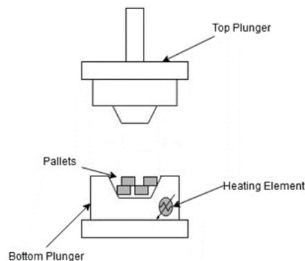
Figure 2.2. Block diagram of hot press compression molding
