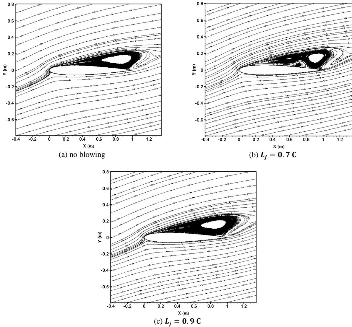
Figure 8. Streamlines at  $I = 0.5$ ,  $\theta = 30^\circ$  and angle of attack  $16^\circ$
