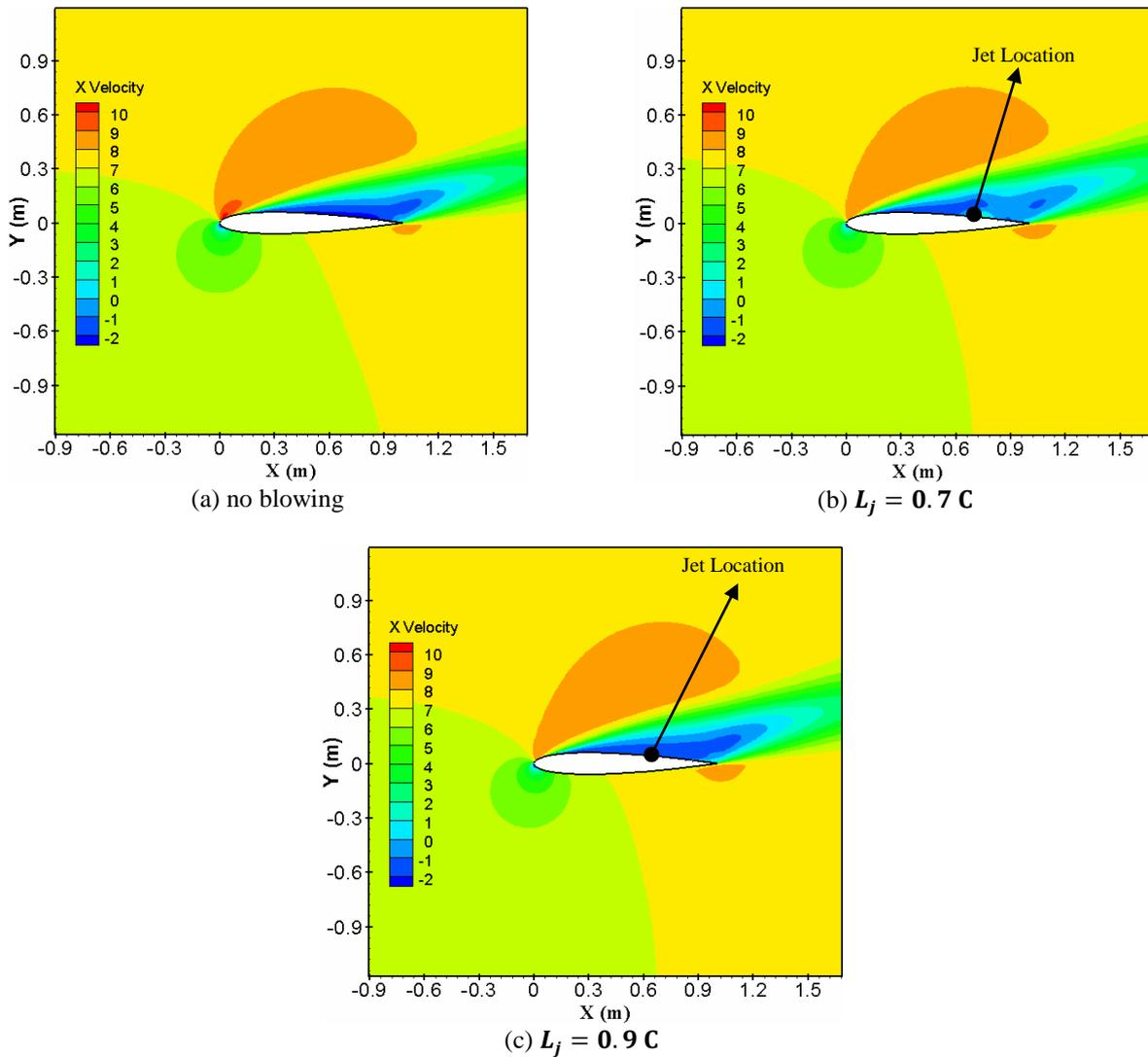
Figure 10. Velocity contour at  $I = 0.5$ ,  $\theta = 30^\circ$  and angle of attack  $16^\circ$
