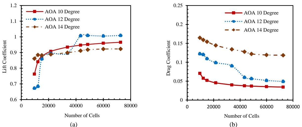
**Figure 2.** Mesh sensitivity analysis for: (a) lift Coefficient and (b) drag coefficient
