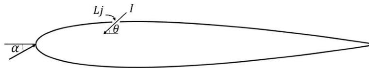
Figure 4. Jet parameters on NACA 0012 airfoil
