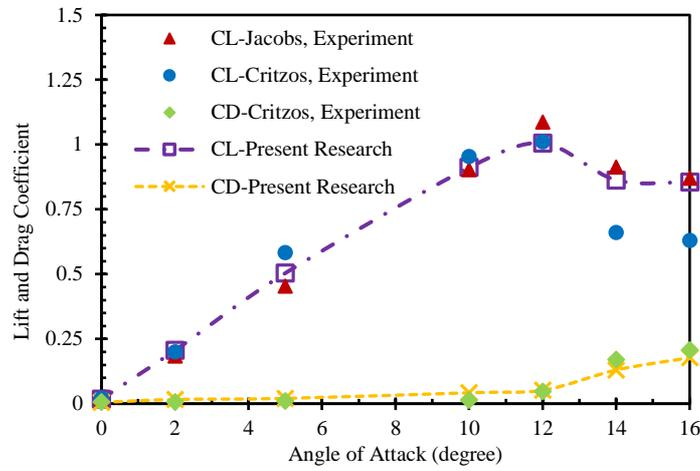
Figure 3. Comparison between numerical and experimental lift and drag coefficients [18, 19].
