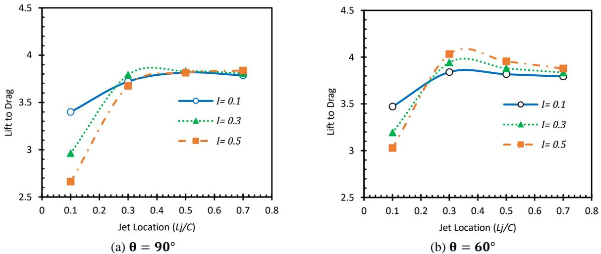
Figure 7. Lift to drag ratio variation at different blowing angles
