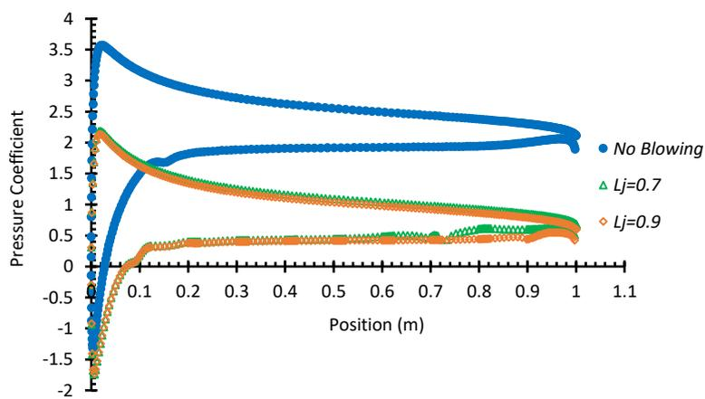
Figure 9. Pressure distribution over airfoil at angle of attack  $16^\circ$
