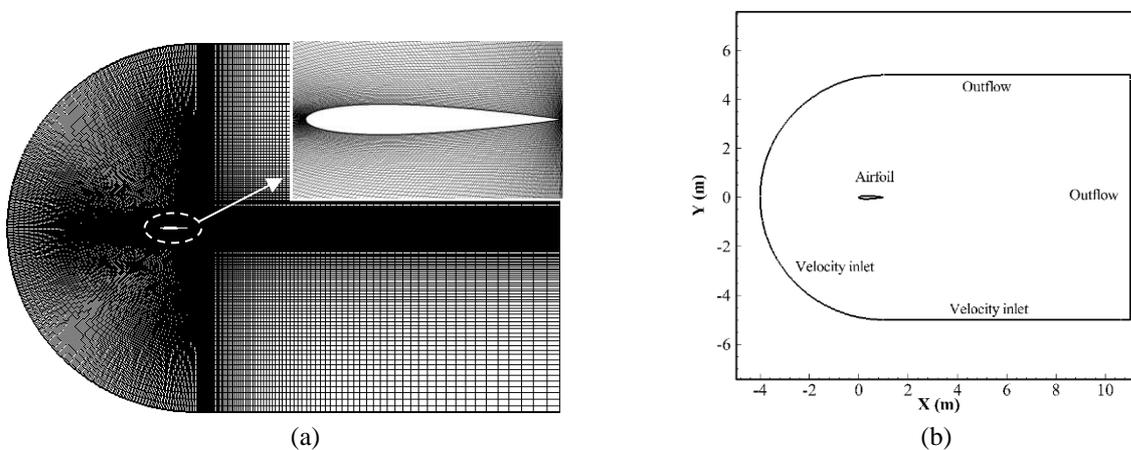
**Figure 1.** (a) Airfoil mesh and (b) boundary conditions of flow over the airfoil
