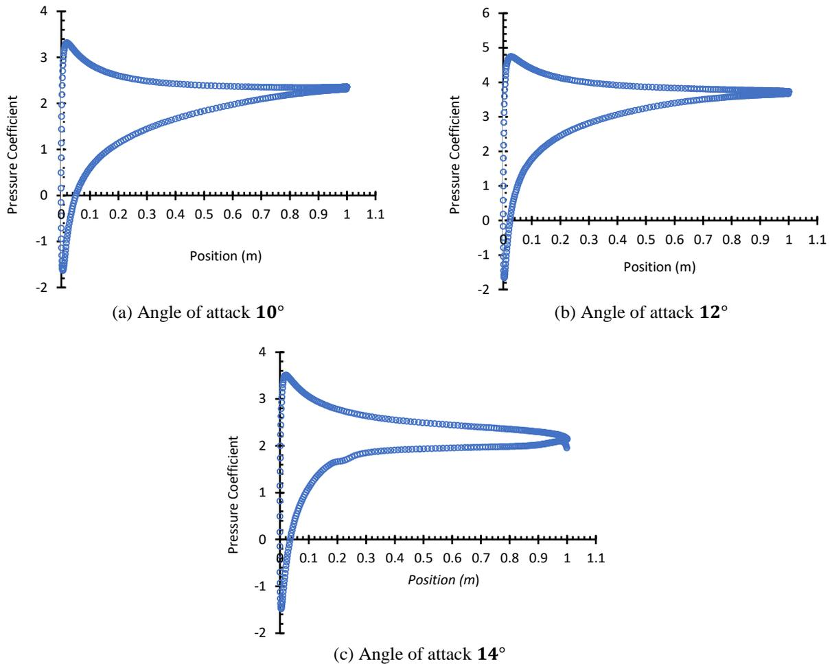
**Figure 5.** Variation of pressure coefficients on the pressure and suction sides of the airfoil
