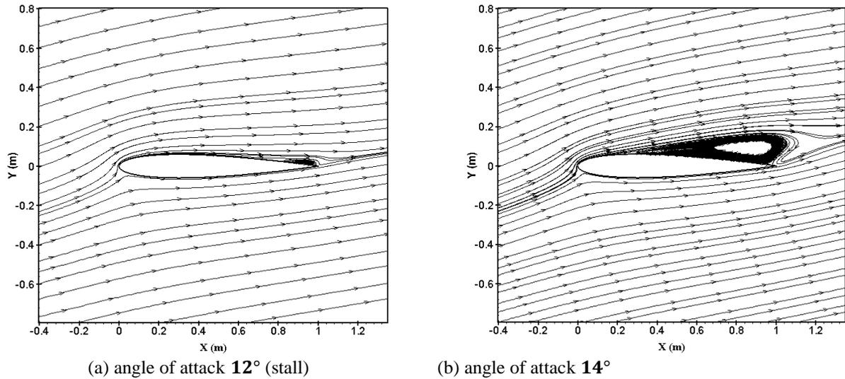
Figure 6. Streamlines over airfoil
