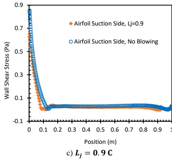
**Figure 11.** Shear stress of airfoil wall on suction side
