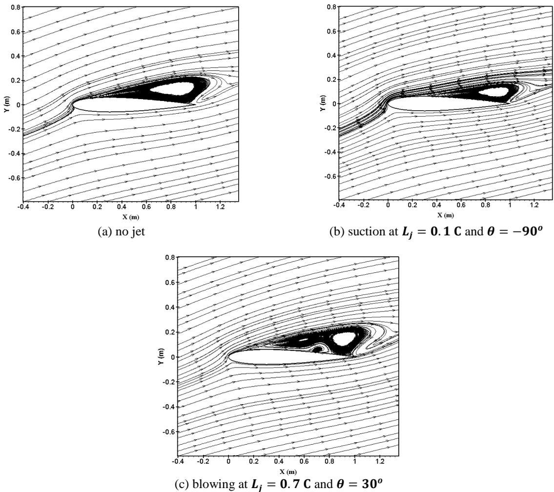
**Figure 12.** Streamlines at  $I = 0.5C$  and angle of attack  $16^\circ$ .
