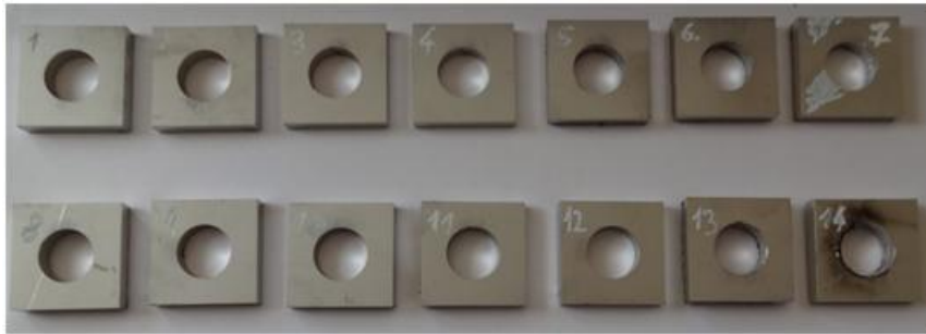
Figure 4. Selected samples cut on fiber laser ( t = 6 mm)
