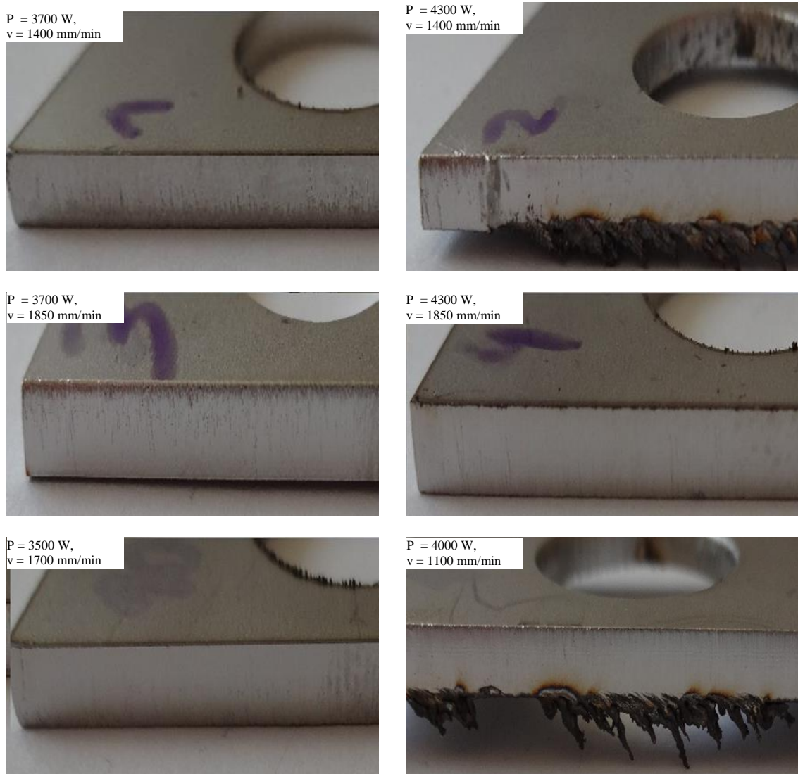
Figure 10. View of sheared edges of selected samples cut on \text{CO}_2 laser ( t = 3 \text{ mm} )
