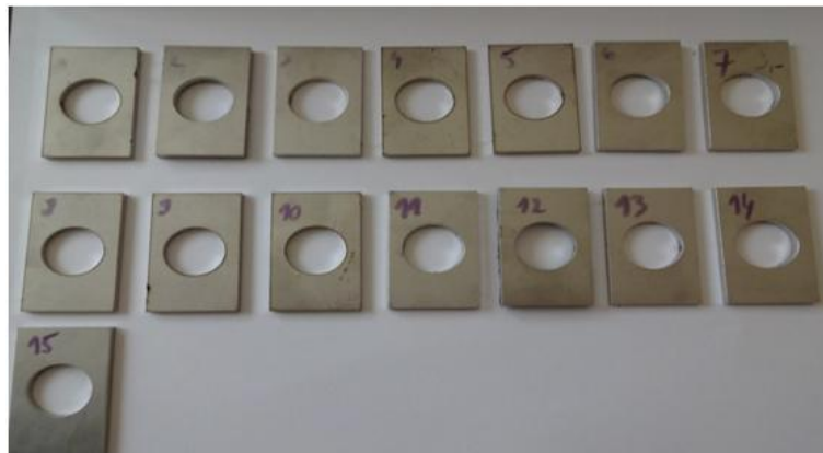
Figure 8. Selected samples cut on a CO 2 laser for t = 3 \text{ mm}
