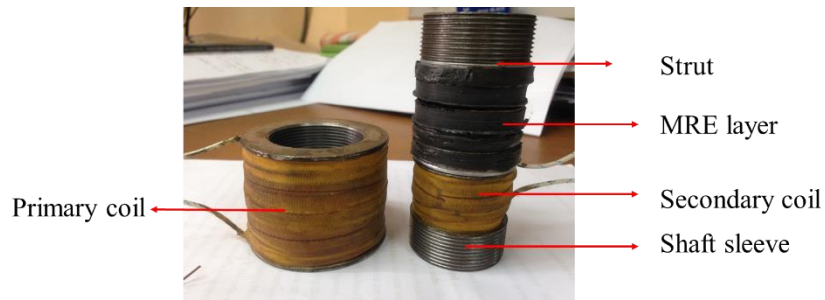
Figure 1(b). Physical structure of the MREID.
