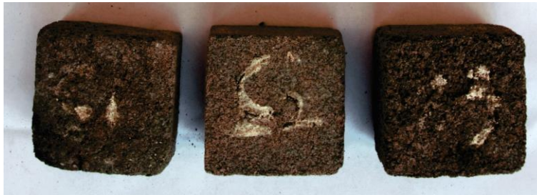
Figure 3. Sintering result of GrC (95-85%) + maize cob powder (5-15%) + 12.5%Na 2 SiO 3 + 12.5%NaOH
