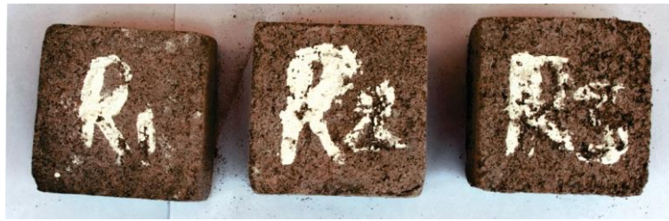
Figure 2. Sintering results of GrC (95-85%) + maize cob powder (5-15%) + 10%Na 2 SiO 3 + 10%NaOH
