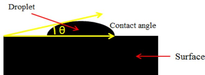
Figure 1. A nanofluid droplet contact angle
