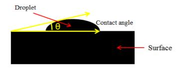
Figure 1. A nanofluid droplet contact angle
