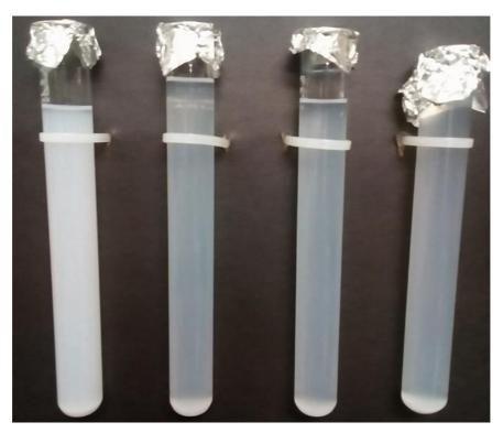
Figure 2. Observation method of nanofluids stability in the test tubes
