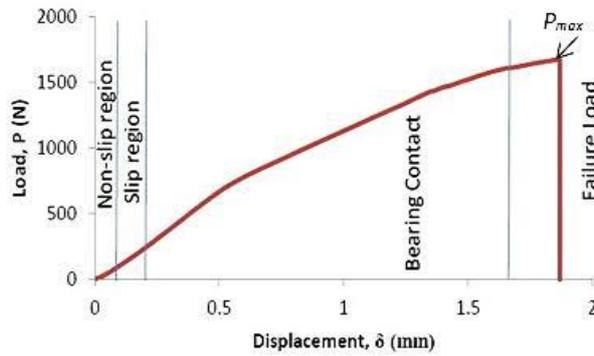
Figure 4. Load-displacement curve profile of PX4 plate in  $W/d = 5$  (taken from [2])
