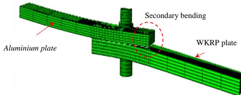
**Figure 4.** The effect of secondary bending in single-lap bolted joints
