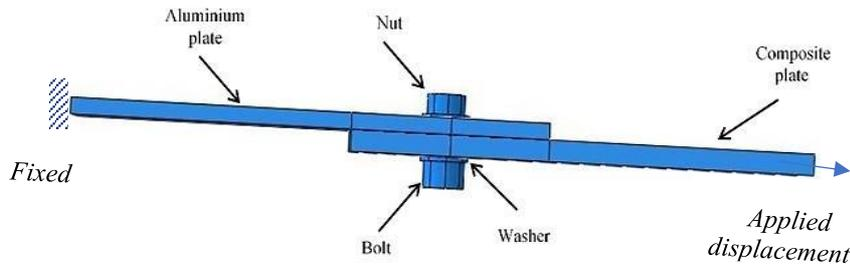
Figure 2. Components in single-lap joint implemented in FEA model
