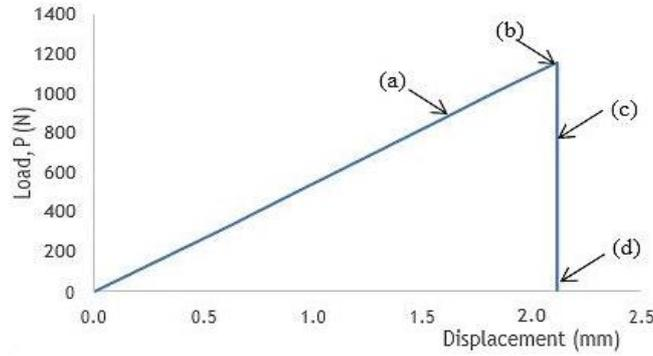
Figure 3. Load-displacement curve profile of PQ4 plate in  $W/d = 5, e/d = 4$
