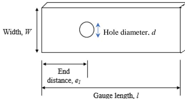
**Figure 1.** Geometries of composite plate used
