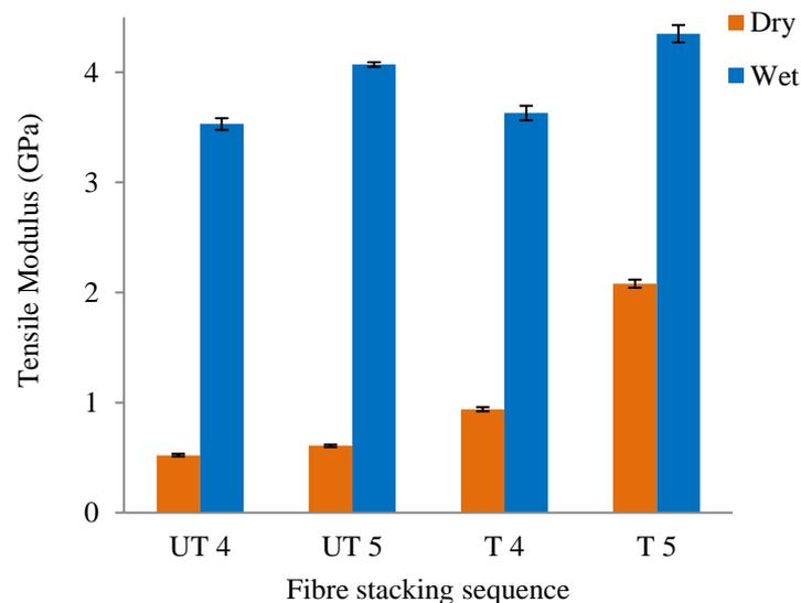
**Figure 5b.** Summary of tensile modulus of dry and wet buri palm fibre reinforced epoxy composites
