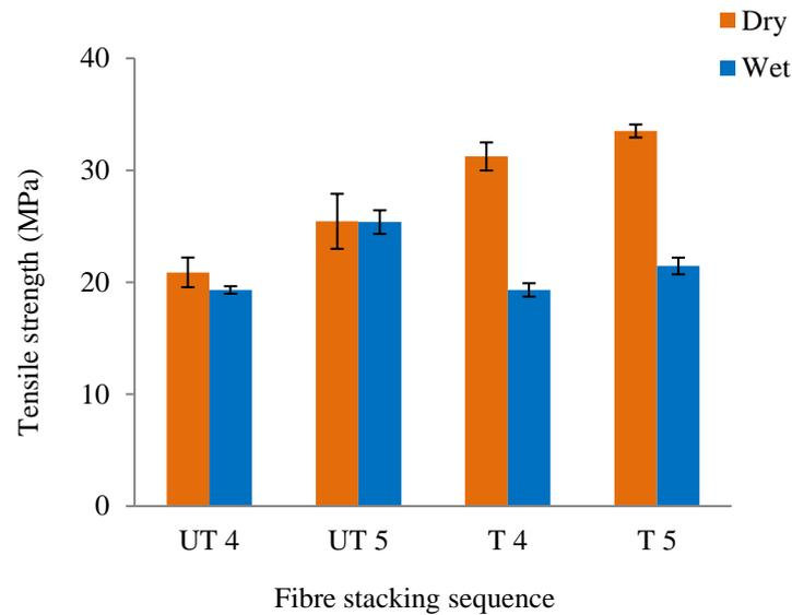
**Figure 5a.** Summary of tensile strength of dry and wet buri palm fibre reinforced epoxy composites
