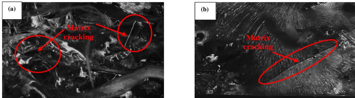
**Figure 7.** Tensile fracture of moisture treated specimen: (a) T4 and (b) T5
