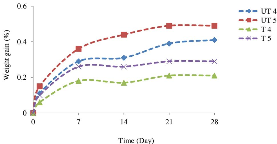
**Figure 3.** Water absorption curves of plain woven sequence stacking laminate composites
