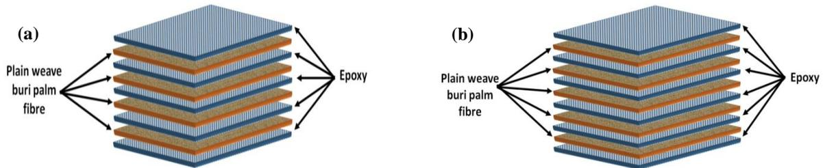
**Figure 2.** Plain woven buri palm fibre reinforced epoxy: (a) 4 layer and (b) 5 layer stacking sequence
