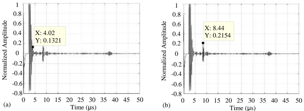
**Figure 1.** Selected points on the graph and calculation of time difference: (a) First echo and (b) Second echo
