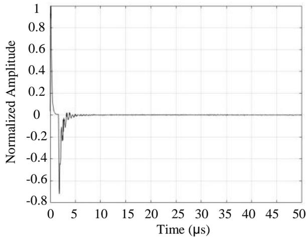
**Figure 6.** Obtained graph from cow’s skin by 10 MHz probe
