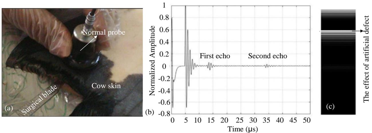
**Figure 8.** Obtained graph from the cow skin with a surgical blade in it by 3.5 MHz probe: (a) Test step, (b) graph obtained in MATLAB program and (c) simulated image in MATLAB
