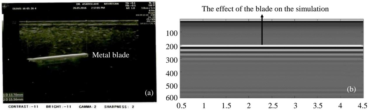
**Figure 13.** Display of the defect level: (a) In ultrasonic and (b) Combining received signals in A-Scan mode
