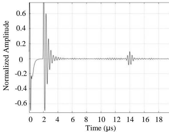
**Figure 5.** Obtained graph from cow’s skin by 3.5 MHz probe
