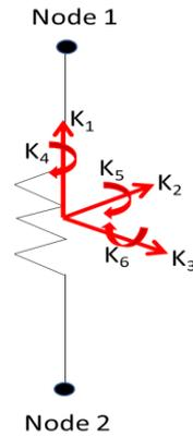
**Figure 4.** Stiffness components of CBUSH
