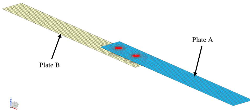
**Figure 2.** FE model of the bolted structure
