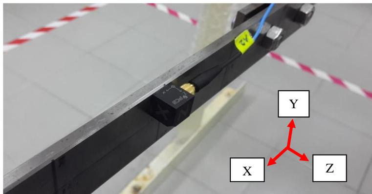
**Figure 6.** Triaxial accelerometer and directions
