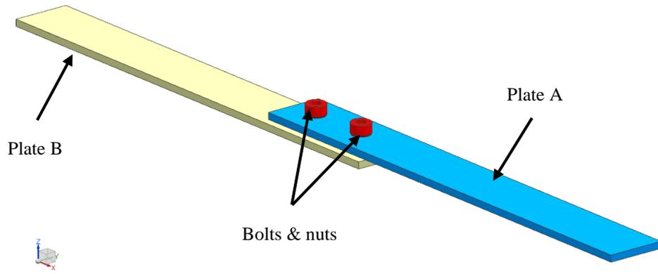
**Figure 1.** 3D CAD model of the bolted structure.
