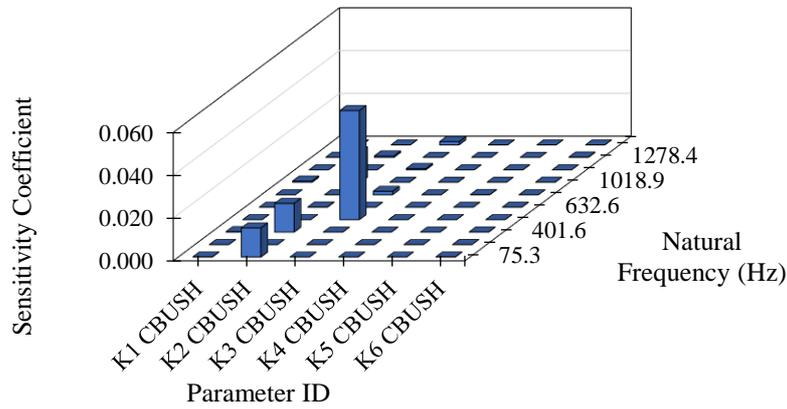
Figure 10. Sensitivity matrix of potential updating parameters
