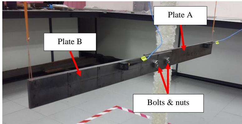
**Figure 5.** Set-up of the bolted joint structure for EMA
