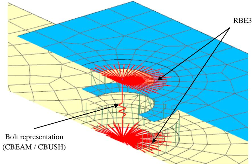
**Figure 3.** Cross-section of the bolted joints
