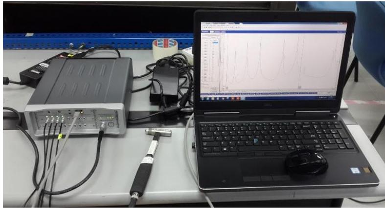
**Figure 7.** Test equipment – LMS Test.Lab and impact hammer
