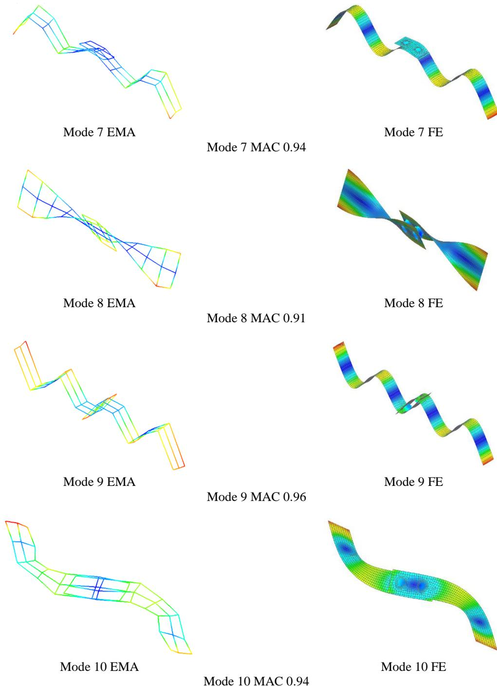
**Figure 9.** Comparison of mode shapes between EMA and FE method with CBUSH element connectors for Mode 6 until Mode 10
