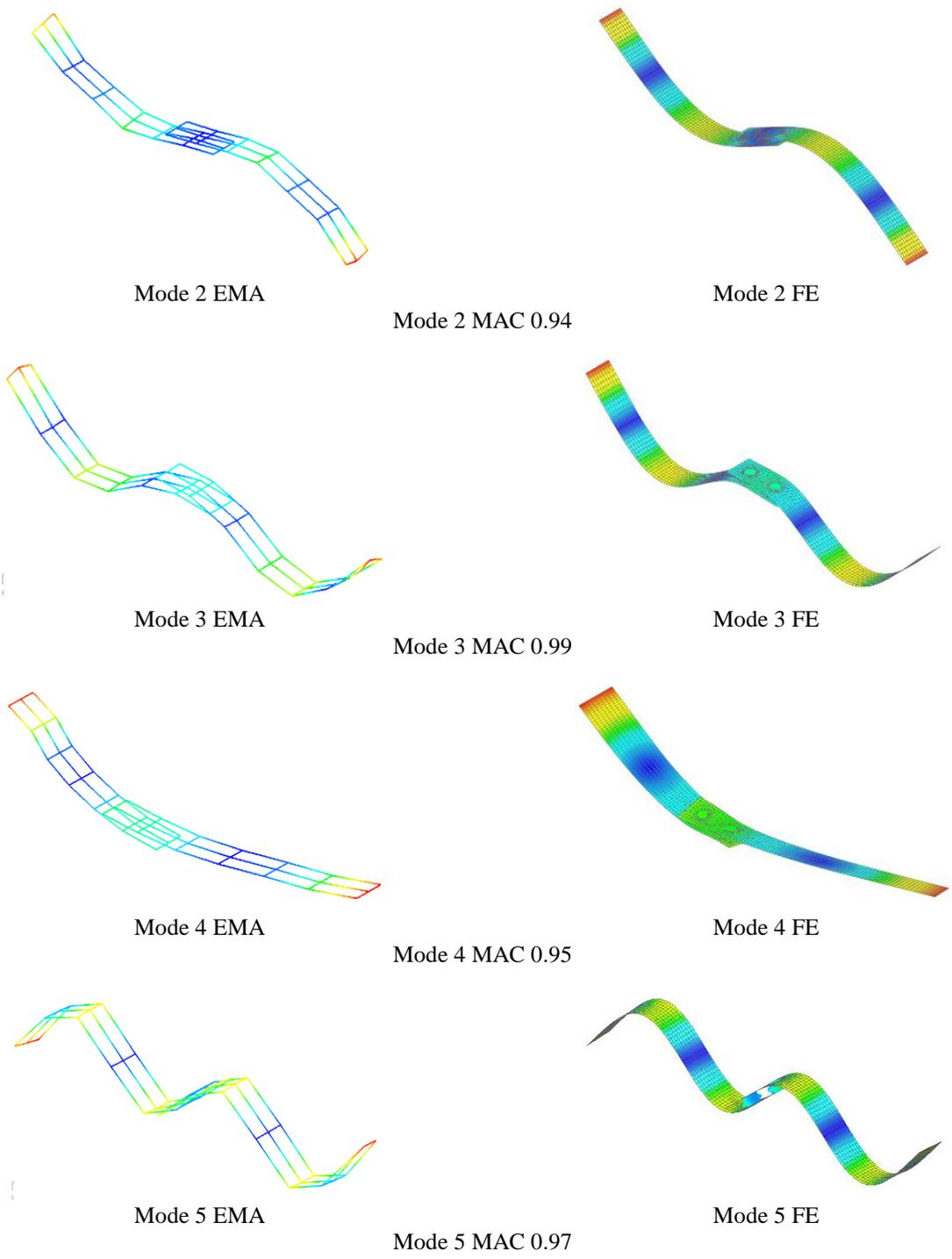
**Figure 8.** Comparison of mode shapes between EMA and FE method with CBUSH element connectors for Mode 1 until Mode 5
