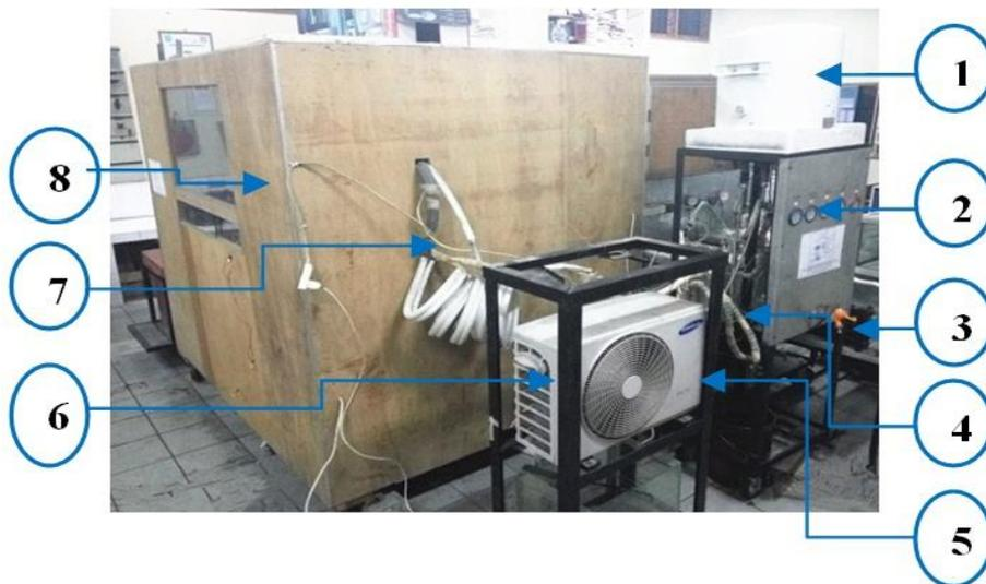
**Figure 2.** Air Source Air Conditioning Water Heater (ASACWH) test apparatus [21].
