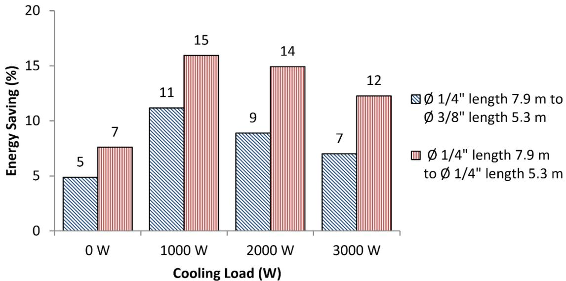
**Figure 9.** Energy-saving of the compressor in ASACWH at various cooling loads in different diameter and length of copper pipe trombone coil.
