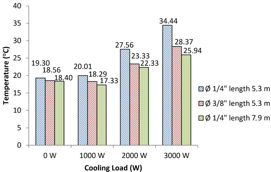
**Figure 6.** Room temperature at various cooling loads in different diameter and length of copper pipe trombone coil.
