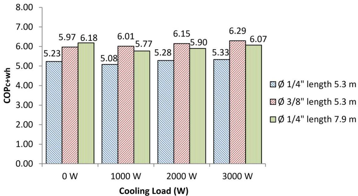
**Figure 11.** The COP<sub>c+wh</sub> (COP cooling and heating of water) in ASACWH at various cooling loads in different diameter and length of copper pipe trombone coil.
