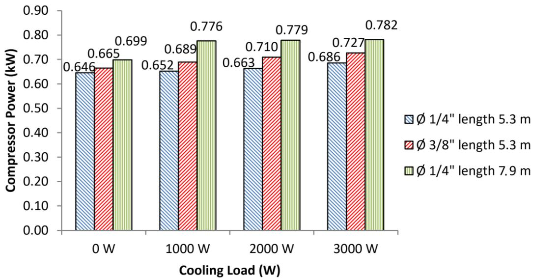
Figure 4. Compressor power at various cooling loads in different diameter and length of copper pipe trombone coil.
