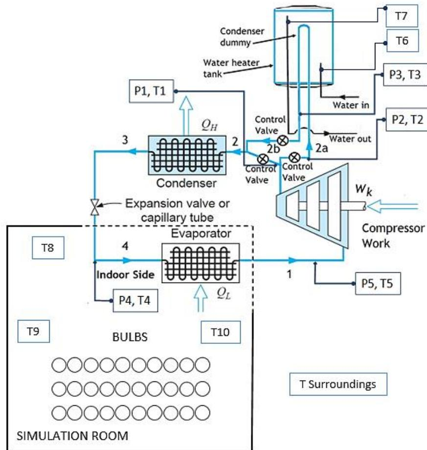
**Figure 1.** Schematic diagram of Air Source Air Conditioning Water Heater (ASACWH) with simulation room at various cooling loads [5].
