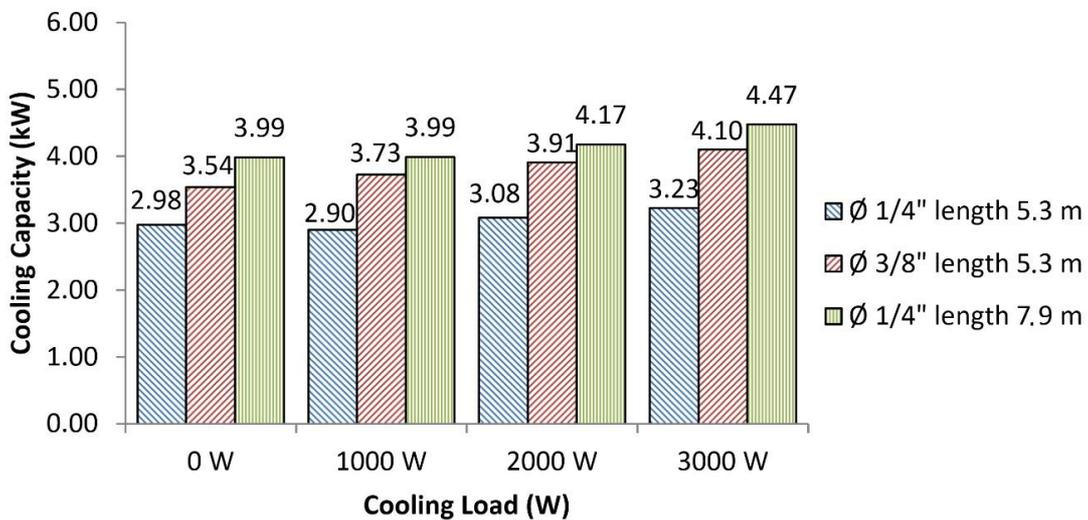
Figure 5. Cooling capacity at various cooling loads in different diameter and length of copper pipe trombone coil.
