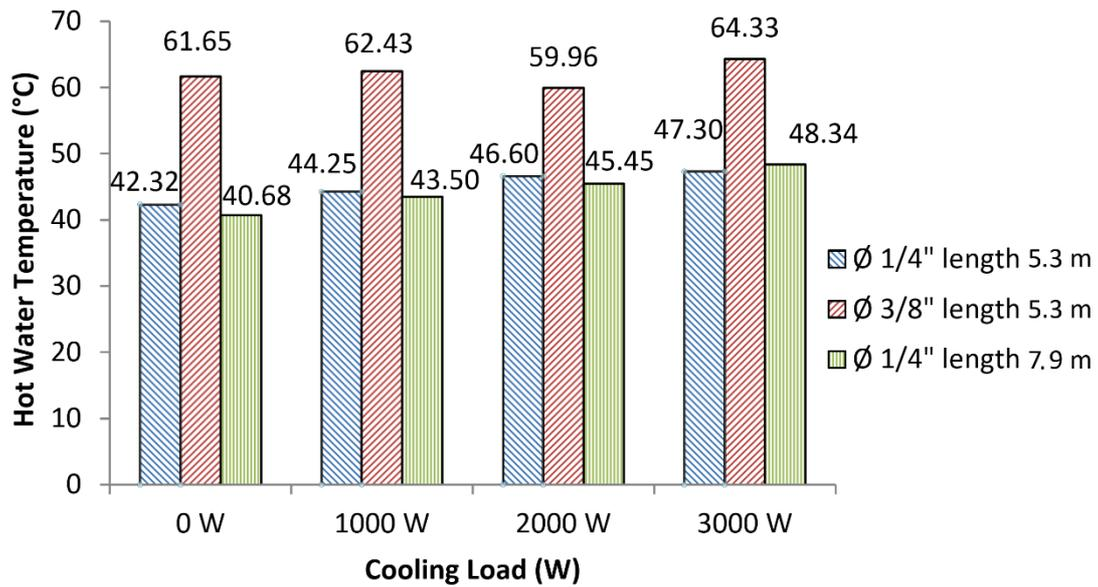
Figure 7. Hot water temperature as a function of cooling load in different diameter and length of trombone coil.
