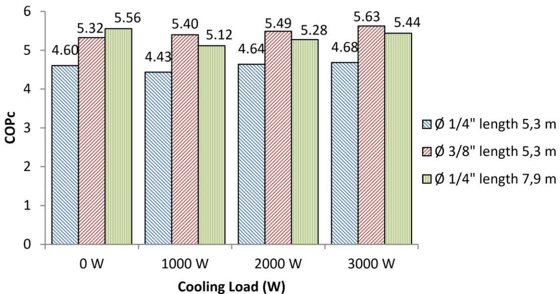
**Figure 10.** The COPc (COP cooling) in ASACWH at various cooling loads in different diameter and length of copper pipe trombone coil.
