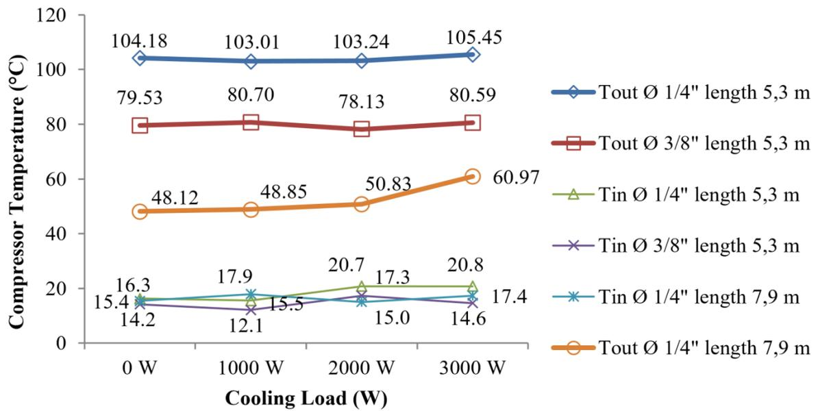
Figure 8. The comparison of suction and discharge temperature of the compressor due to the cooling load in different diameter and length of copper pipe trombone coil.
