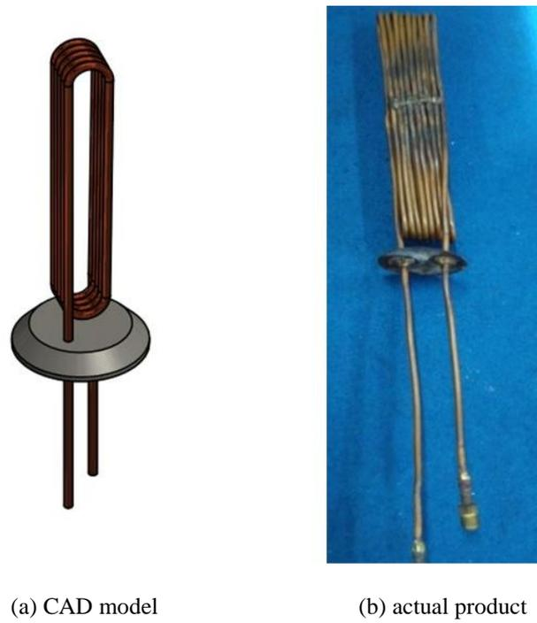
**Figure 3.** Trombone coil as dummy condenser: (a) CAD model [23] and (b) actual product [24].
