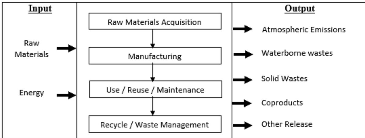
**Figure 1.** System boundary of hybrid oil palm/glass fibre-reinforced polyurethane composites for automotive crash box using manufacturing pulforming process [29]
