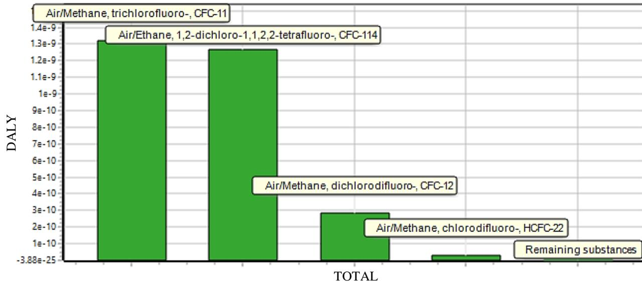
**Figure 5.** Ozone depletion damage assessment of pulforming process per impact categories results using oil palm/glass fibre-reinforced Polyurethane composite for ACB.
