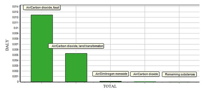
Method: ReCiPe Endpoint (H) V1.13 / Europe ReciPe H/A / Damage assessment / Excluding long-term emissions. Analyzing 1 kg Oil Palm Natural/Gas Fiber Reinforced Polyurethane Hybrid Composite for ACB.
