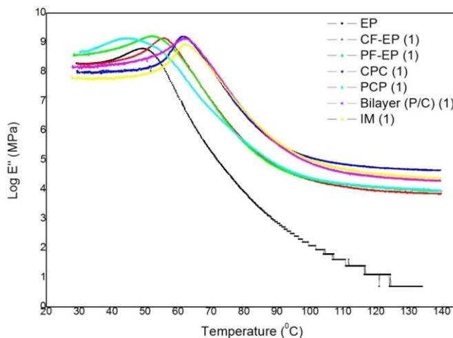
**Figure 7.** Effect of layering pattern and fiber hybridization with temperature on the loss modulus of fabricated composites at a frequency of 1 Hz
