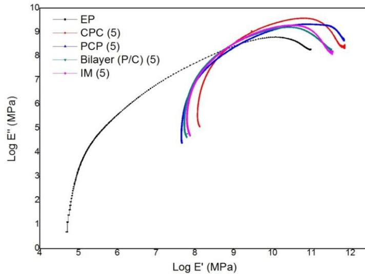
**Figure 13.** Cole-Cole plots of neat epoxy and hybrid composites at a frequency of 5 Hz
