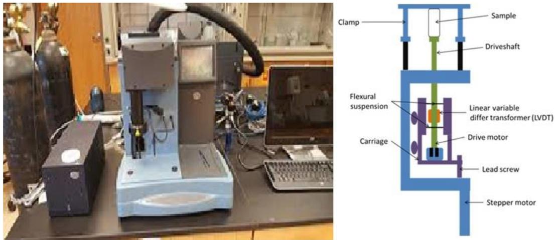
Figure 4. DMTA Q800 test instrument
