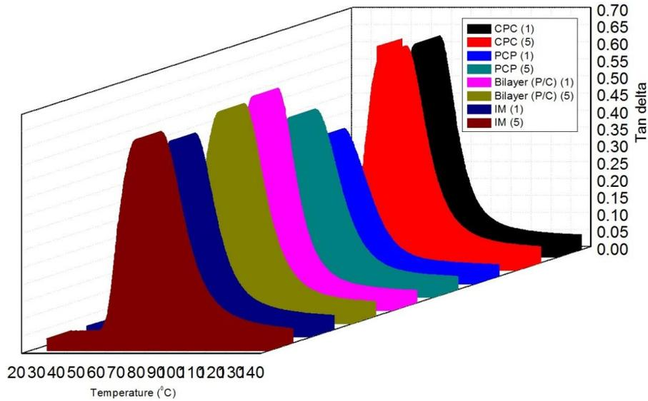
**Figure 11.** Three dimensional thermogram of different layered PALF/COIR hybrid epoxy composites
