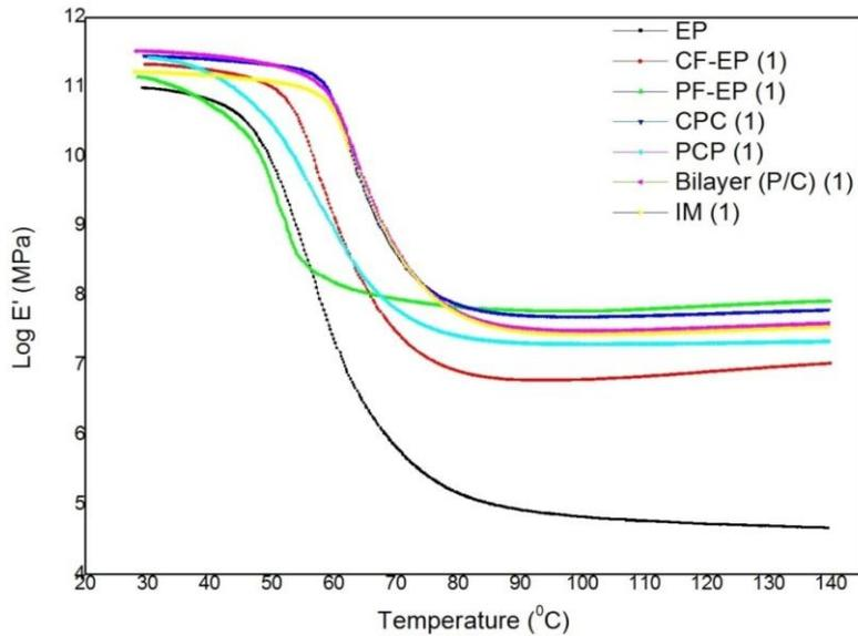
**Figure 5.** Effect of layering pattern and fiber hybridization with temperature on the storage modulus of fabricated composites at a frequency of 1 Hz
