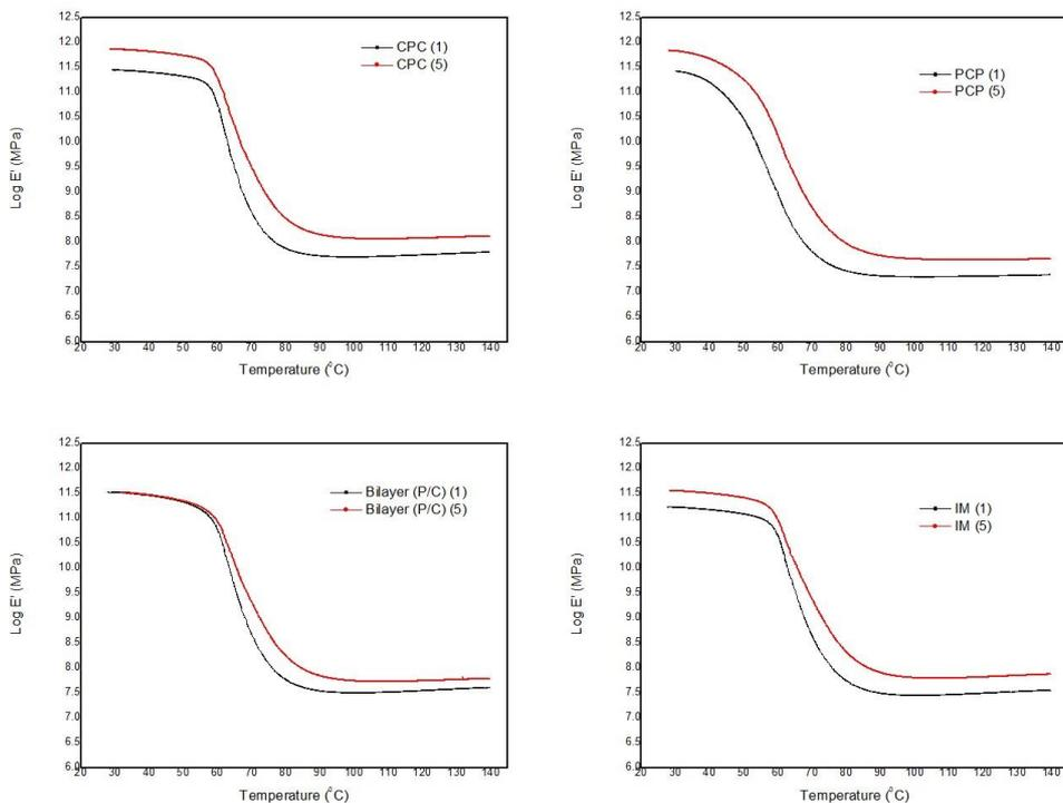
**Figure 8.** Effect of frequency with temperature on the storage modulus of fabricated hybrid composites
