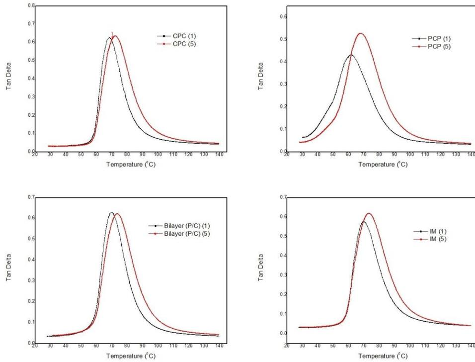
**Figure 9.** Effect of frequency with temperature on the damping ratio ( $\tan \delta$ ) of fabricated hybrid composites
