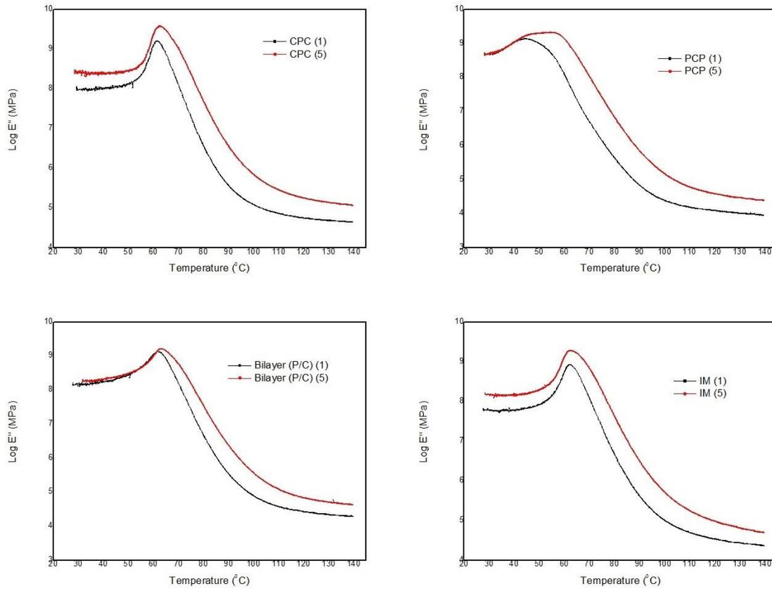
**Figure 10.** Effect of frequency with temperature on the loss modulus of fabricated hybrid composites
