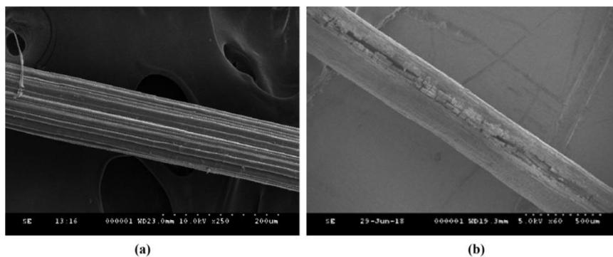
**Figure 1.** Surface morphology of (a) PALF and (b) COIR
