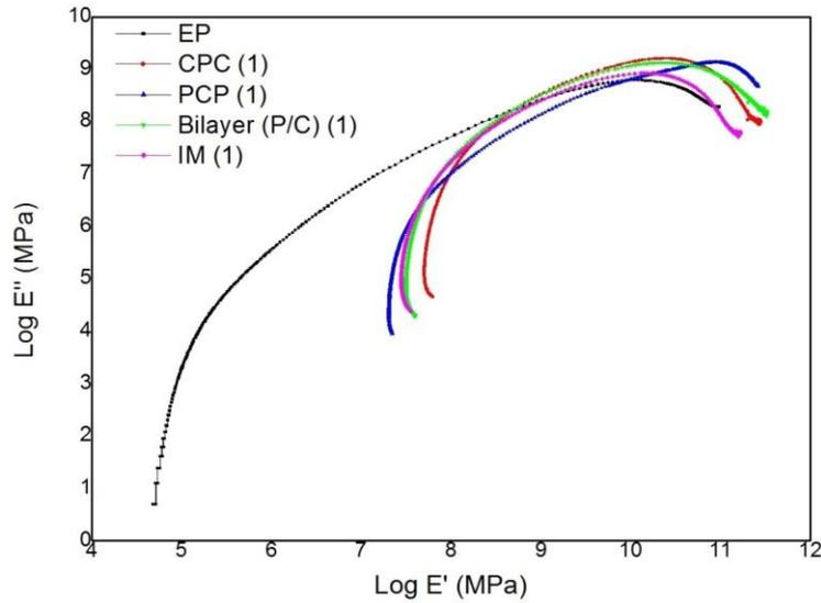
**Figure 12.** Cole-Cole plots of neat epoxy and hybrid composites at a frequency of 1 Hz
