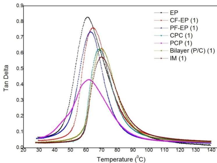
**Figure 6.** Effect of layering pattern and fiber hybridization with temperature on the loss damping factor ( $\tan \delta$ ) of fabricated composites at a frequency of 1 Hz
