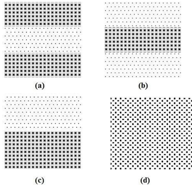
**Figure 2.** Different layering pattern of hybrid composites (a) PCP, (b) CPC, (c) Bilayer (P/C) and (d) IM
