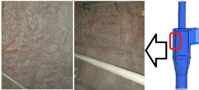
**Figure 5.** Erosion on cyclone wall at cylindrical section
