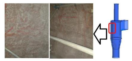
Figure 5. Erosion on cyclone wall at cylindrical section
