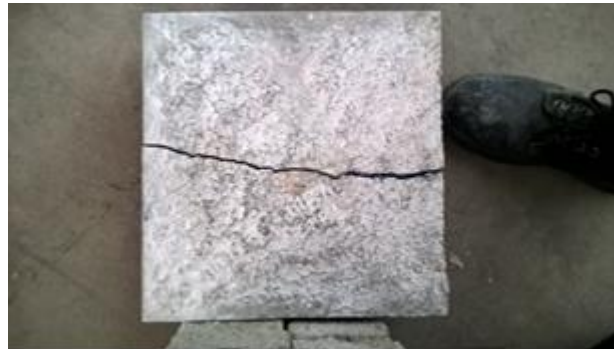
Figure 9. Crack pattern for batch 1.
