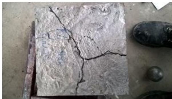
Figure 10. Crack pattern for batch 2.
