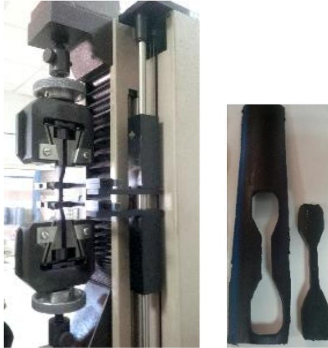
Figure 1. Machine and standard specimen for tensile test
