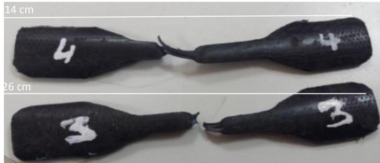
Figure 3. Example of broken specimens after the tensile test.
