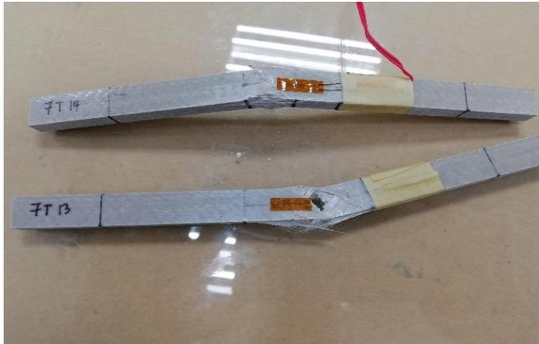
**Figure 10.** Top view of failed-composite coupon sample
