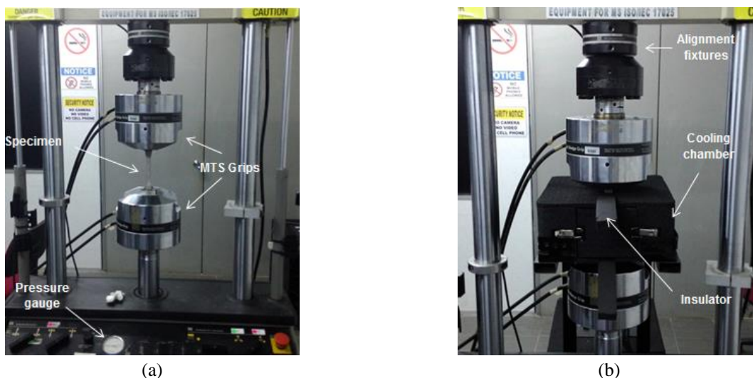
Figure 1. MTS 810 servo hydraulic machine set up at: (a) room temperature and (b) low temperature
