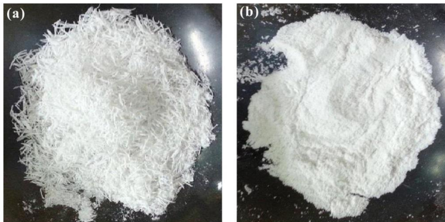
Figure 1. RHA particle: (a) before ground and sieved and (b) after ground and sieved
