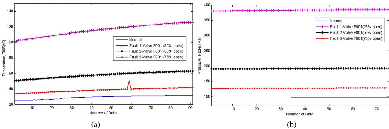
Figure 10. Fault model for hot-heat exchanger: (a) output T005 and (b) output P004
