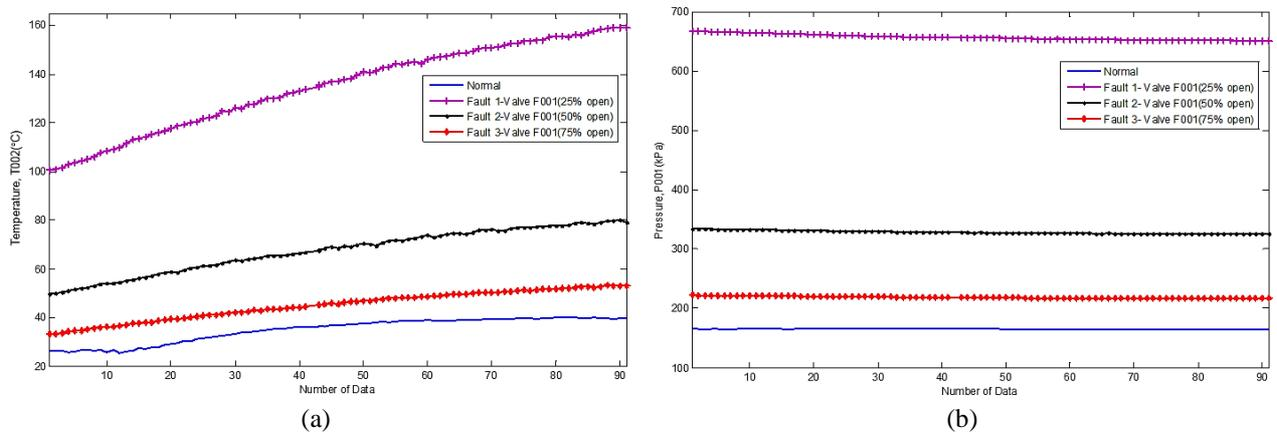
Figure 12. Fault model for reactor: (a) output T002 and (b) output P001
