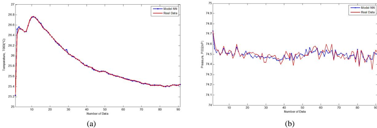
**Figure 7.** ANN modelling for cold-heat exchanger: (a) output T003 and (b) output P002
