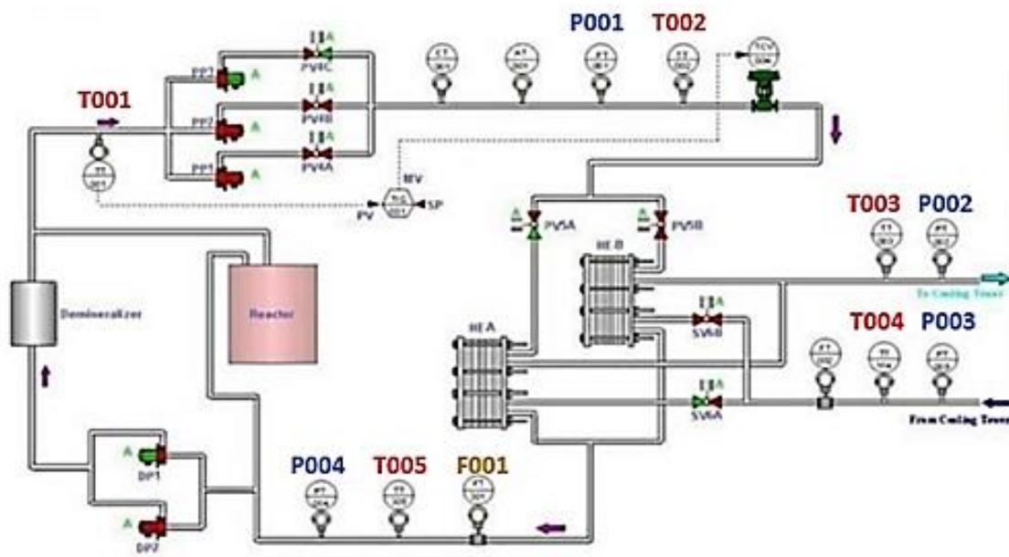
Figure 1. SCADA of the primary and secondary cooling system for RTP
