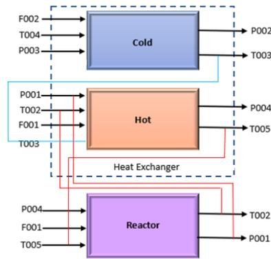
**Figure 4.** Block diagram of RTP cooling system
