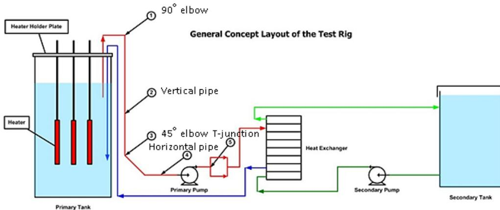
Figure 2. The schematic diagram for the simulated experimental test rig
