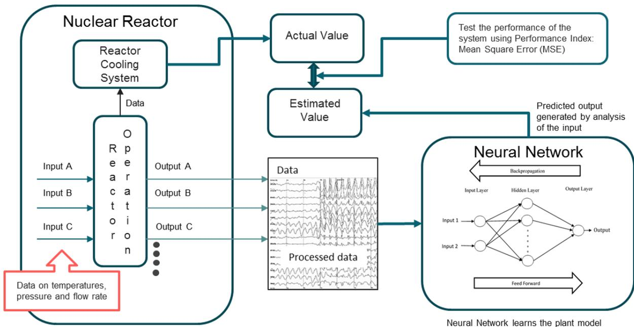
Figure 3. Plant model with a neural network
