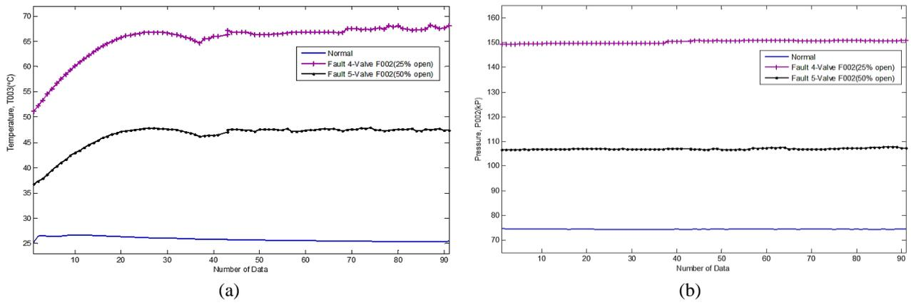
Figure 11. Fault model for cold-heat exchanger: (a) output T003 and (b) output P002
