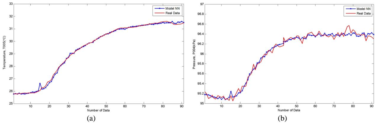
Figure 8. ANN modelling for hot-heat exchanger: (a) output T005 and (b) output P004
