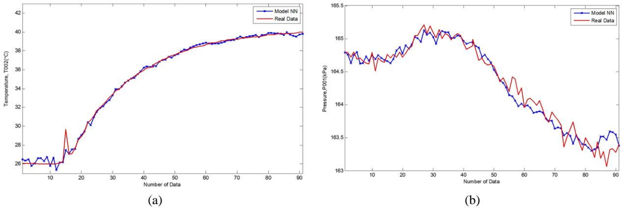
Figure 9. ANN modelling for reactor: (a) output T002 and (b) output P001
