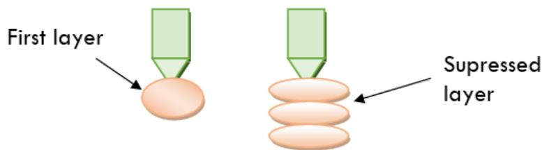
**Figure 11.** The first layer and suppressed layer of the small hole diameter
