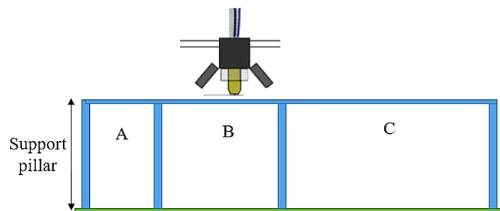
**Figure 9.** Fabrication of multiple overhang length using 3D printer
