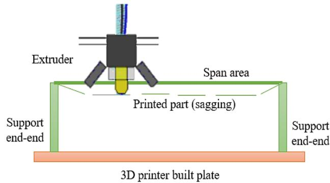
**Figure 8.** Process diagram of bridge fabrications using a 3D printer
