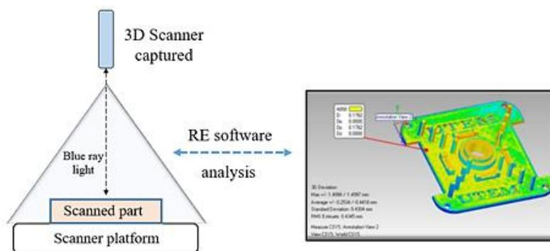
**Figure 4.** Schematic diagram of scanning process
