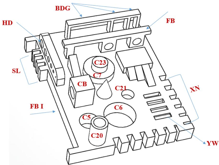
**Figure 2.** CAD model representation on benchmarking artifact
