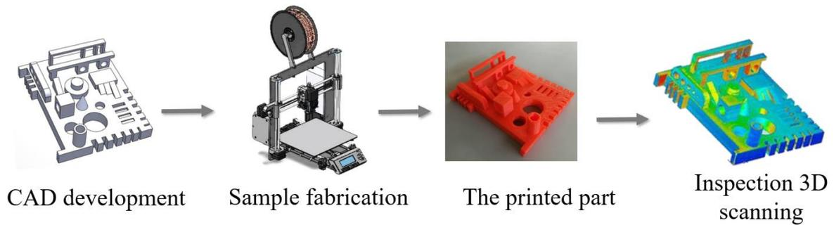
**Figure 1.** The process flow in experimental fabrication and inspection of dimensional accuracy
