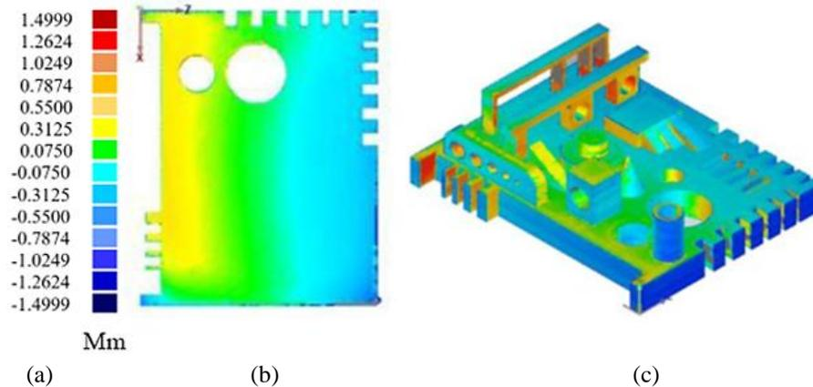
**Figure 5.** (a) Color segment (b) Error map analyses of benchmarking artifacts in back view (c) Error map analyses of benchmarking artifacts in isometric view
