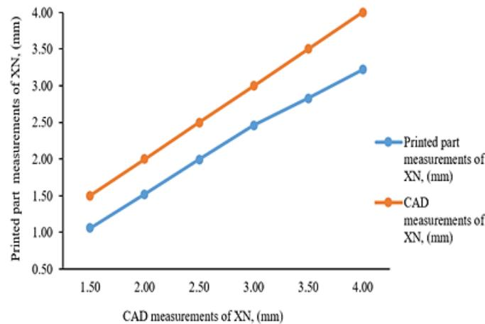
**Figure 6.** Printed parts and CAD measurements of XN, (mm)
