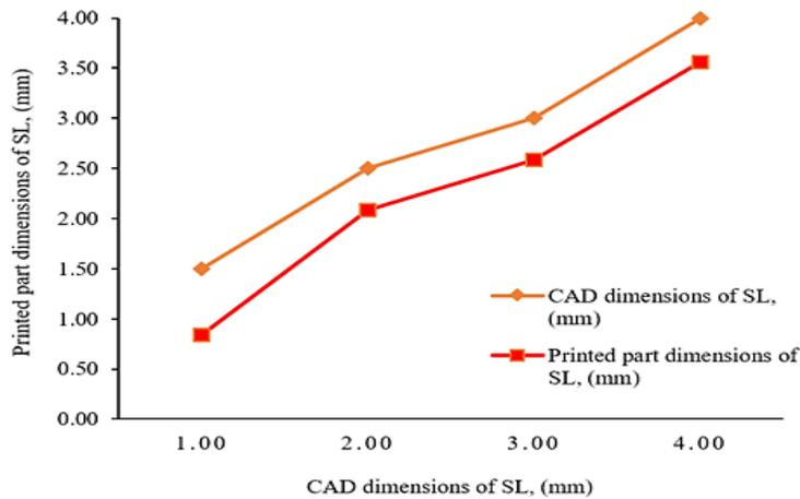
Figure 7. CAD and printed parts measurements of SL, (mm)
