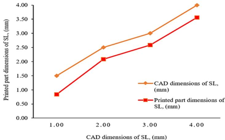
Figure 7. CAD and printed parts measurements of SL, (mm)
