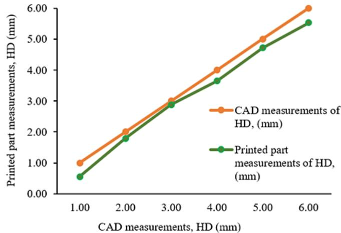
**Figure 10.** Printed part and CAD measurements of HD, (mm)
