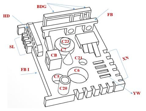
Figure 2. CAD model representation on benchmarking artifact
