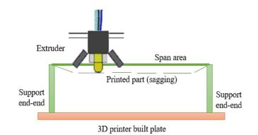
Figure 8. Process diagram of bridge fabrications using a 3D printer
