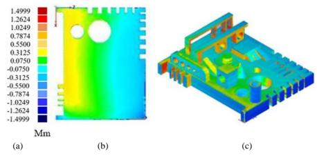
Figure 5. (a) Color segment (b) Error map analyses of benchmarking artifacts in back view (c) Error map analyses of benchmarking artifacts in isometric view
