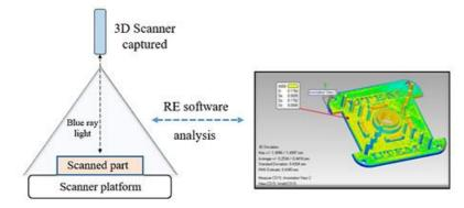
Figure 4. Schematic diagram of scanning process
