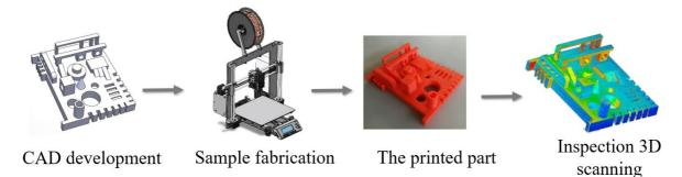
Figure 1. The process flow in experimental fabrication and inspection of dimensional accuracy
