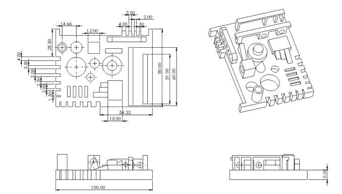
Figure 3. The detail measurements of benchmark artifacts
