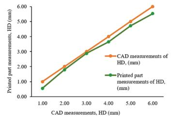
Figure 10. Printed part and CAD measurements of HD, (mm)
