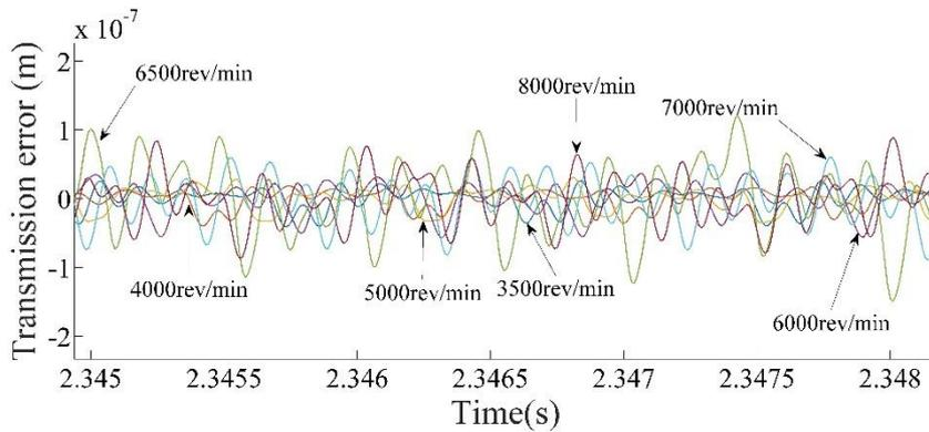
**Figure 8(a).** Transmission error vs time for different load and speed
