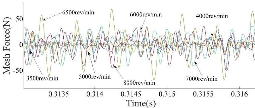
Figure 6. Mesh force vs time for different load and rotational speed
