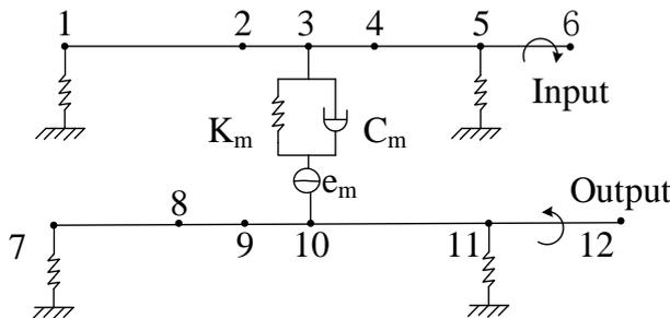
Figure 3. Finite element model for overall system
