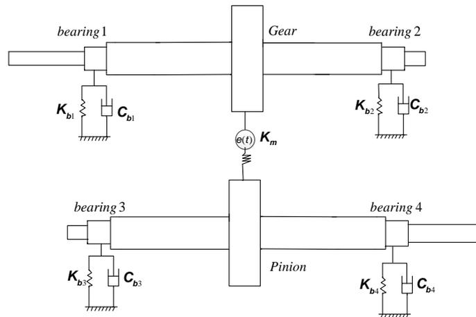
Figure 1. Single stage structure for gear transmission system
