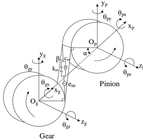
**Figure 2.** 12 DOF dynamic model of a helical gear pair
