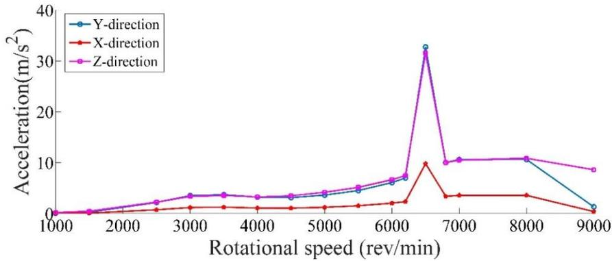
Figure 5. Acceleration response map along X, Y and Z-direction at Node 1 for different speeds
