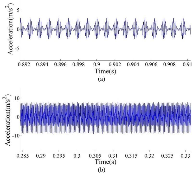
**Figure 4.** Vibration acceleration for different rotational speeds at node 3: (a) 3000 rev/min and (b) 9000 rev/min
