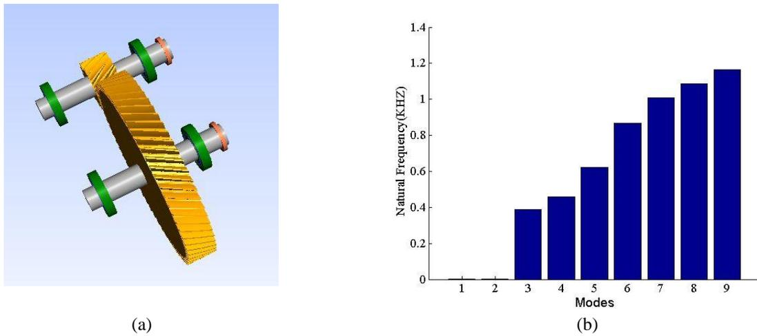
Figure 9. (a) MASTA 3-D model and (b) damped natural frequencies
