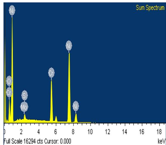
Figure 9. EDX for NCM composite.
