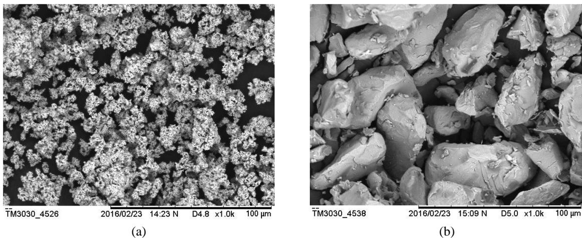
**Figure 1.** (a) Powder morphology of nickel and (b) Powder morphology of chromium.
