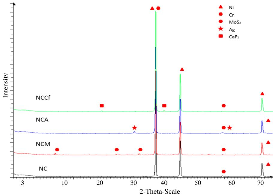
**Figure 14.** XRD analysis of Ni-Cr composites before sintering.
