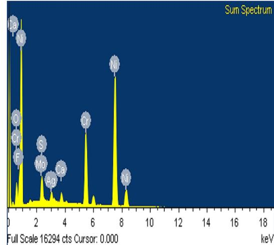
**Figure 13.** EDX of NCCf composite.**Table 5.** Elemental composition in NCCf composite.
