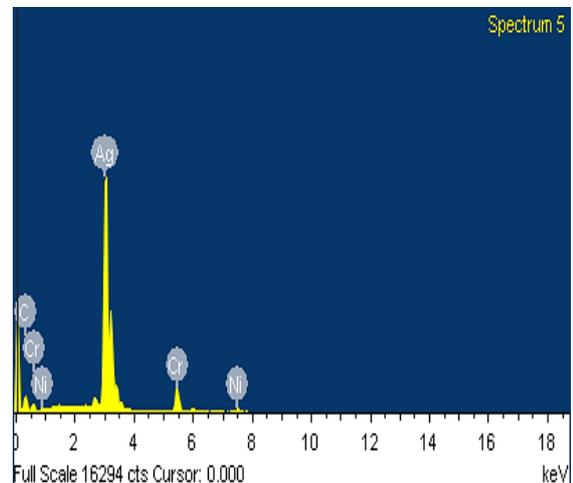
Figure 11. EDX of NCA composite on white phase.
