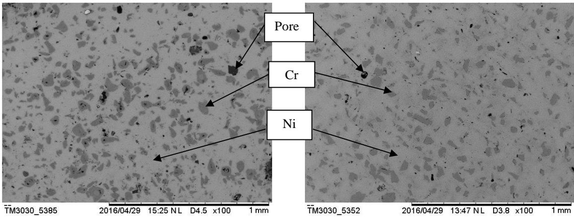
Figure 6. NC sintering at 1000°C.
