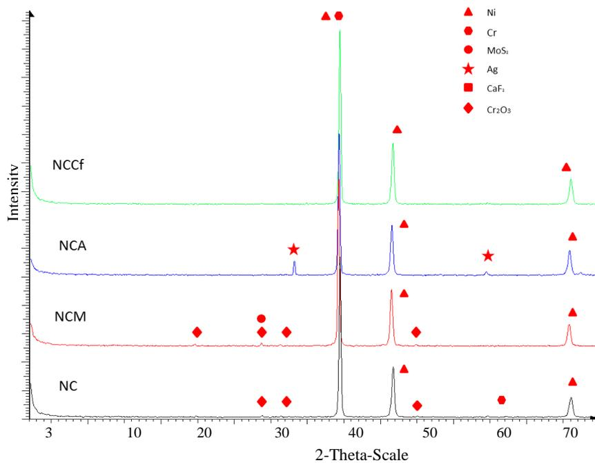
**Figure 15.** XRD analysis of Ni-Cr composites after sintering.
