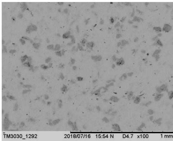
Figure 8. SEM micrograph of NCM composite.
