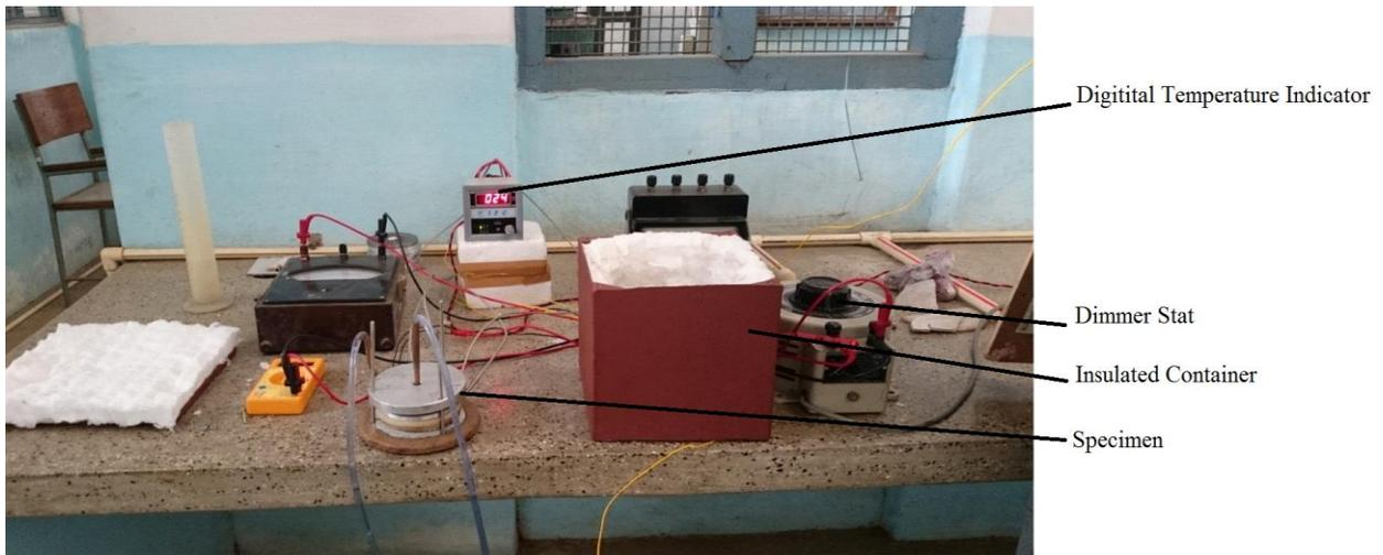
Figure 3. Experimental setup used for measurement of thermal conductivity of composite.
