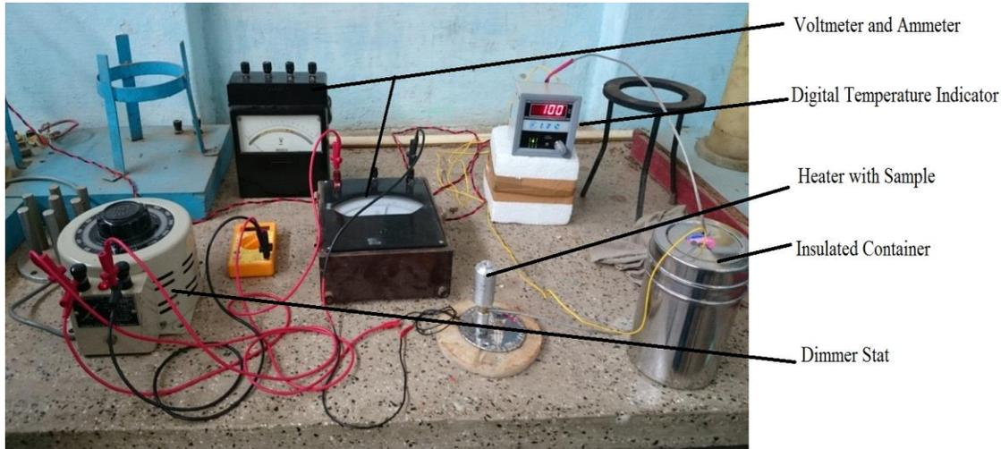
Figure 2. Experimental setup used for the measurement of specific heat capacity.
