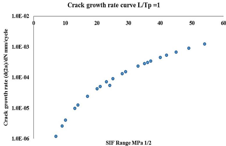
Figure 8. Comparison of SIF and rate of crack growth ( $L/T_p=1$ ).
