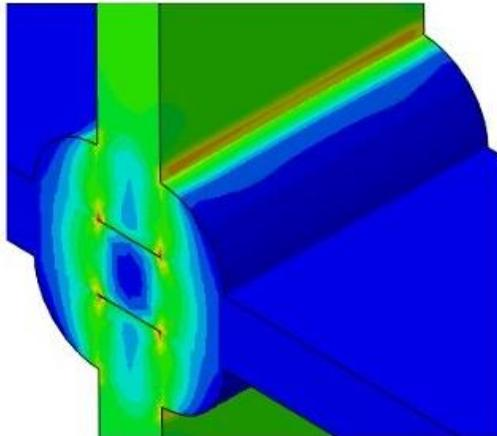
Figure 10. 3D model of cruciform weld shape (convex).
