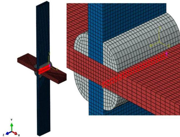
Figure 11. Meshing of convex shape weld joint.
