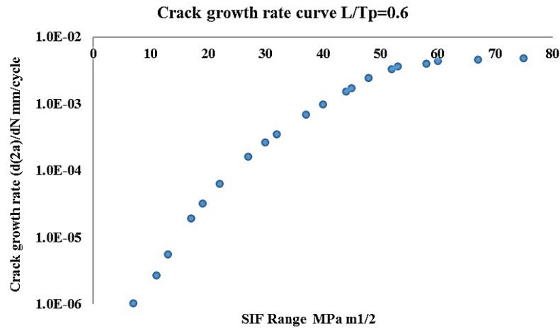
Figure 9. Comparison of SIF and rate of crack growth ( $L/T_p=0.6$ ).
