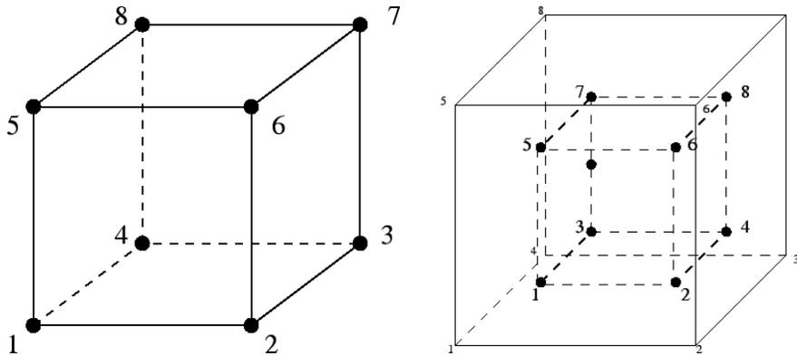
Figure 4. Noded Brick element with Reduced Integration (C3D8R).
