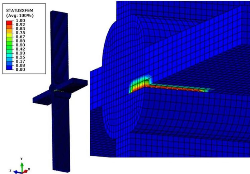
(a) Crack propagation at step 3
