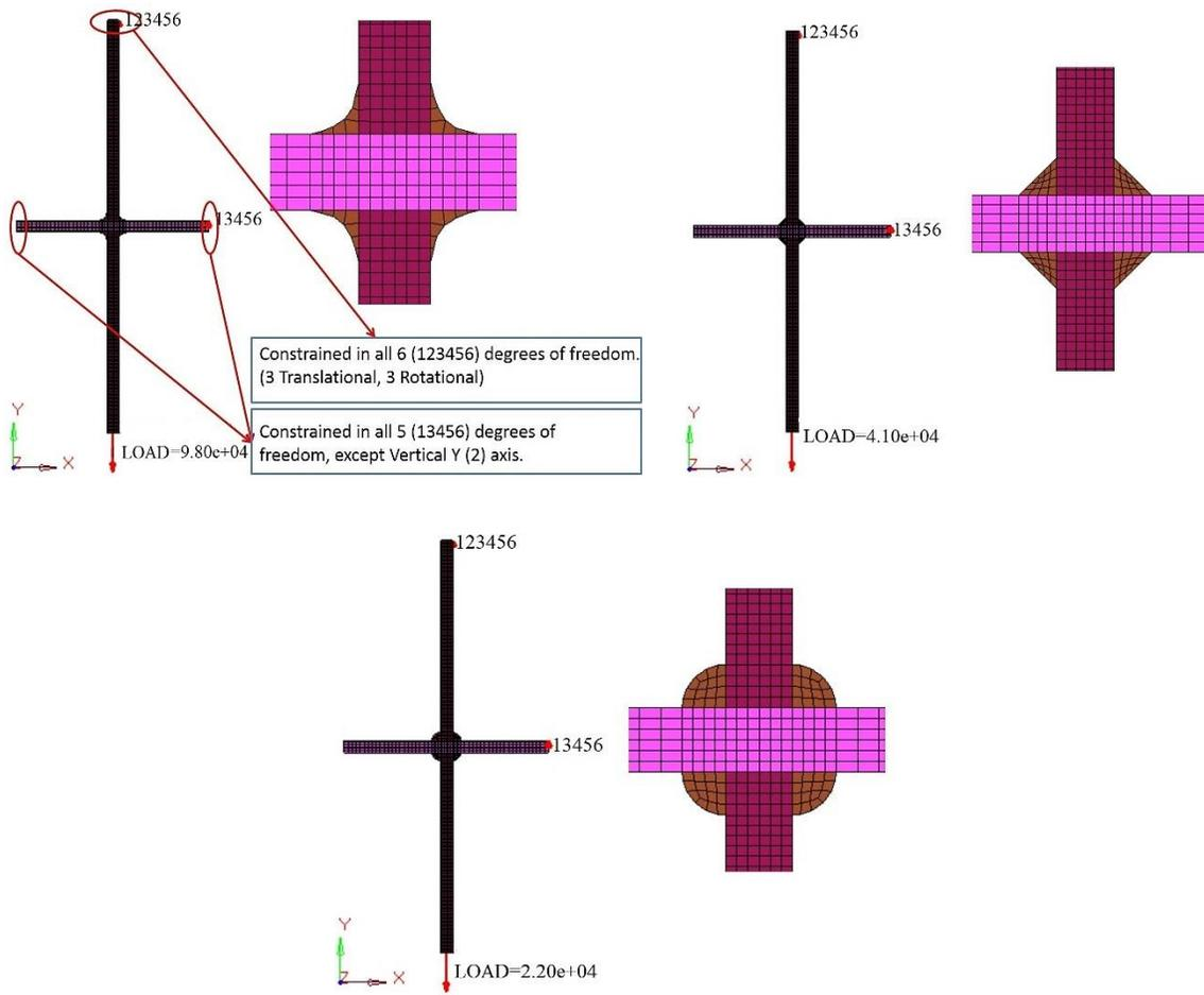
Figure 5. Boundary conditions for concave, flat and convex shape specimen.
