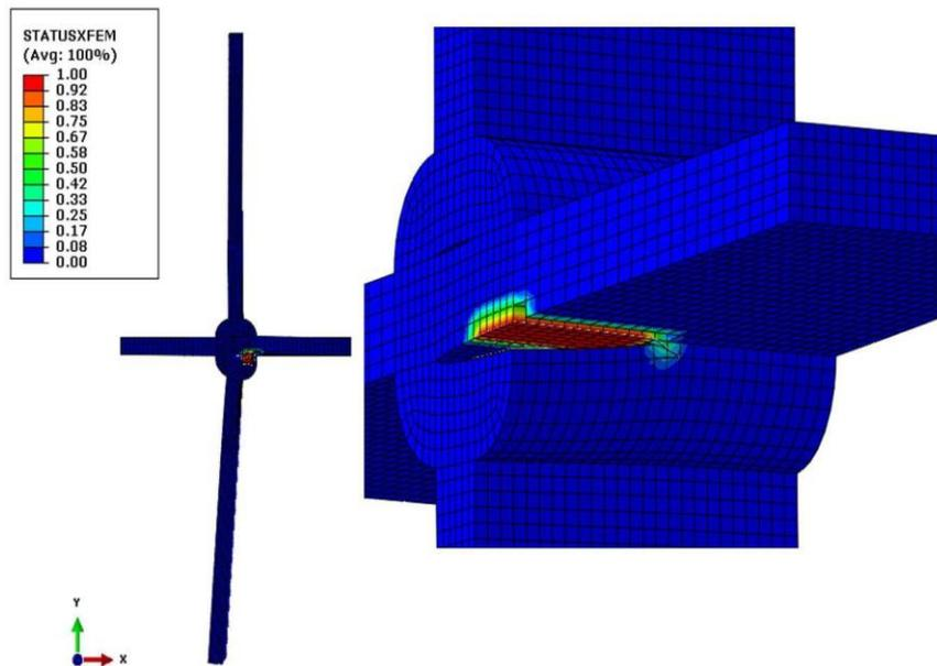
(b) Crack propagation at step 6
