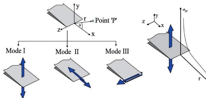
Figure 3. Modes of failure [16].
