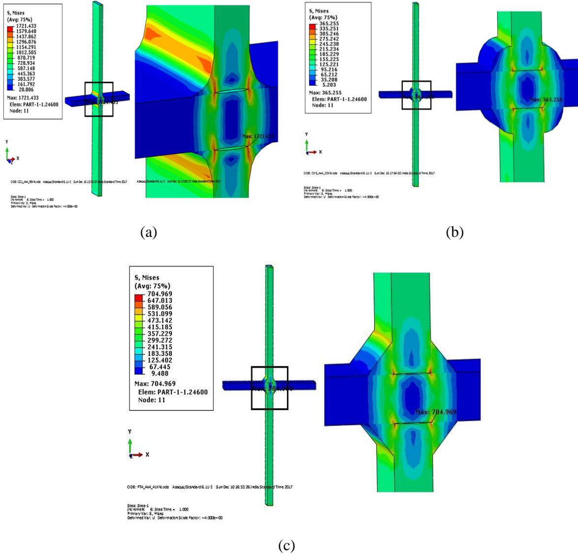
Figure 6. Static analysis of cruciform weld joints of different weld bead shapes (a) Concave specimen, (b) Convex shape specimen and (c) flat weld shape.
