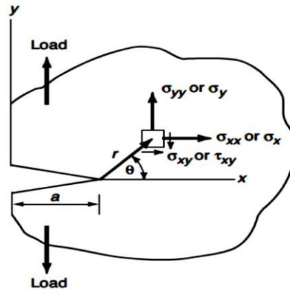
Figure 2. Stresses observed in co-ordinate system to the front of the crack [16].
