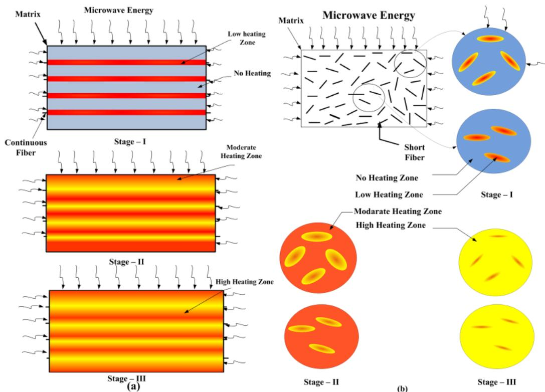
**Figure 7.** Microwave heating of polymer composite with (a) continuous fibers and (b) short fibers.
