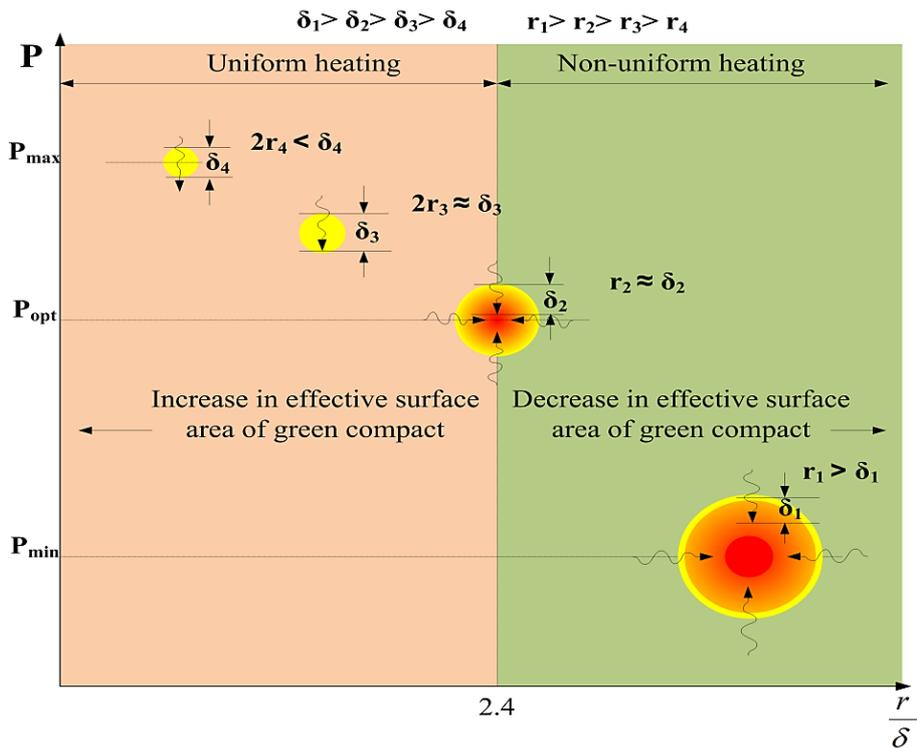
Figure 6. Microwave heating of non-magnetic metal.
