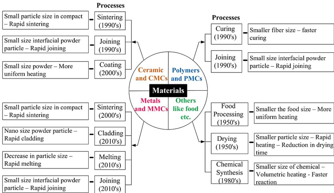
Figure 2. Effects of material size in various applications of microwave processing.
