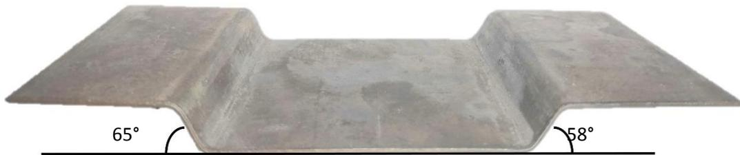
Figure 8. Bending angles of sheet metal by hot press forming experiment.
