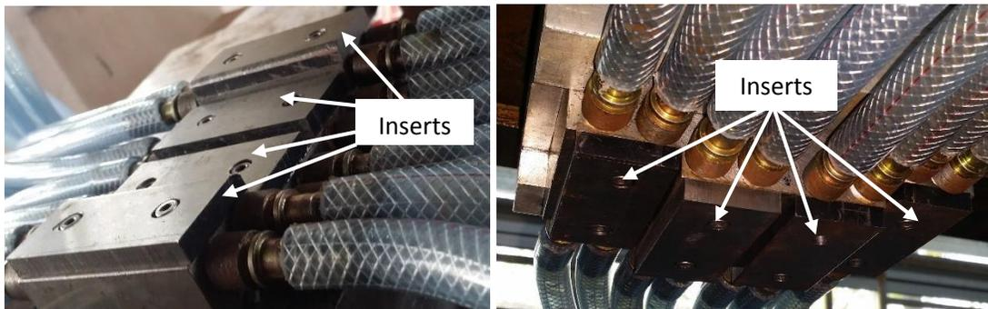
Figure 2. Inserts installed on the punch and die.
