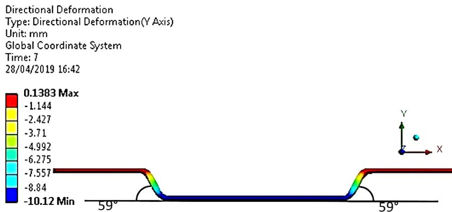
Figure 9. Bending angles of sheet metal by ANSYS transient structural.
