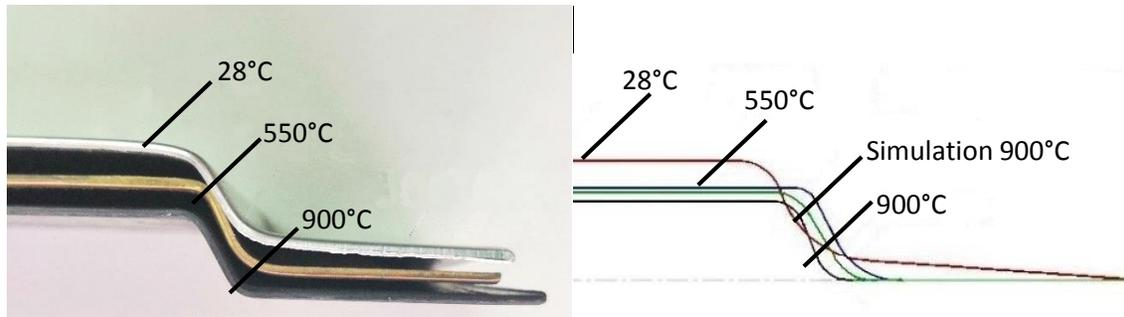
Figure 7. Bending angle of workpieces under different pre-heating temperature.
