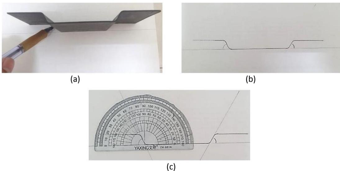
Figure 5. Procedures of measuring the bending angles of stamped workpiece: (a) tracing the bending profile, (b) sketched bending profile, (c) measuring of bending angles.
