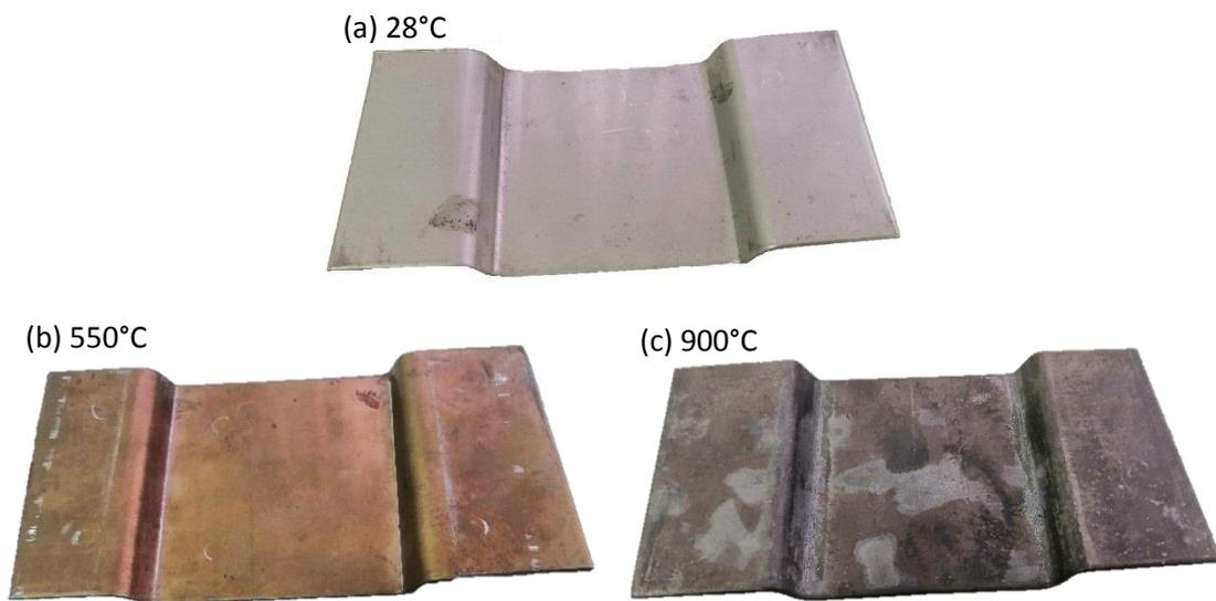
Figure 6. As-formed part under different pre-heating temperature.
