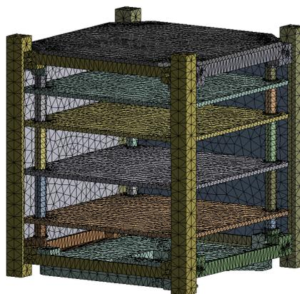
Figure 3. MYSat meshing configuration in ANSYS
