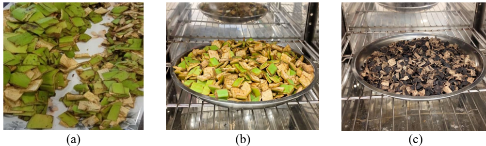
Figure 1. Drying process step: (a) BPs were cut into small pieces, (b) BPs were placed in the oven, and (c) Oven-dried BPs
