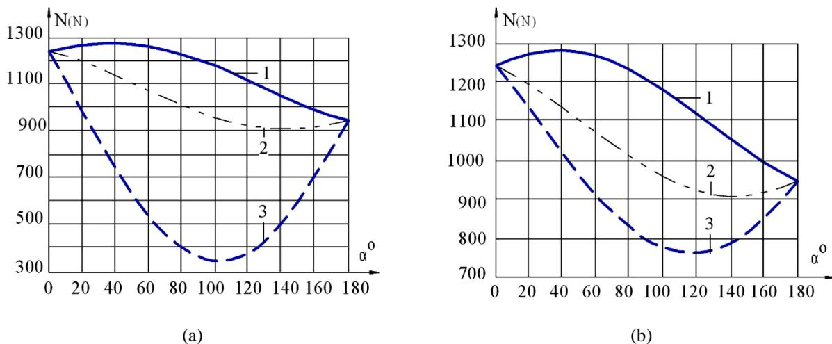
**Figure 5.** Graphs of technological reaction change  $N = f(\alpha)$  depending on the robot travel surface inclination angle  $\alpha$  to the horizon at a friction coefficient of the robot grips: (a)  $\mu = 0.2$  and (b)  $\mu = 0.5$ .
