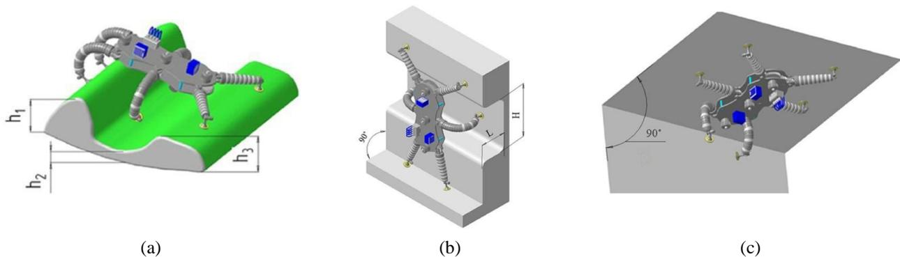
**Figure 3.** Options of the position of the mobile robot when moving on surfaces of arbitrary orientation.
