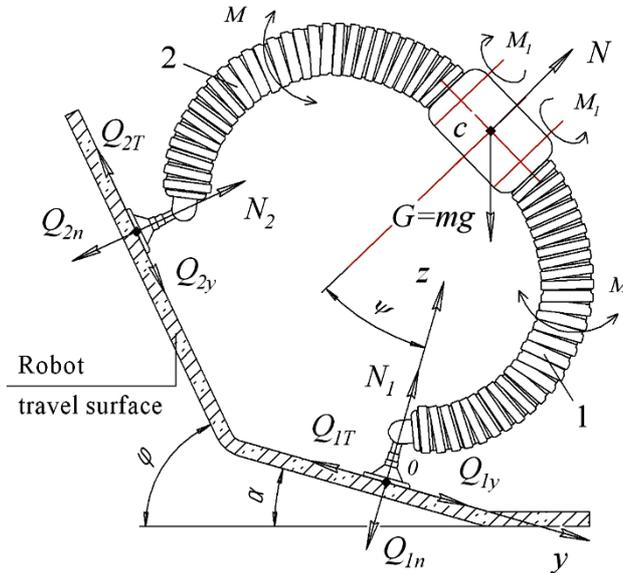
**Figure 4.** The scheme of forces acting on the robot.
