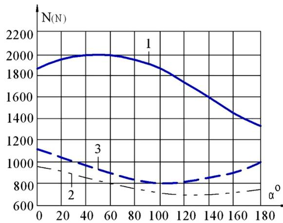
**Figure 6.** Graphs of technological reaction change  $N = f(\alpha)$  with the difference in the slope of the surfaces on which the robot legs rest  $\varphi - \alpha = 30^\circ$  and with a friction coefficient of the robot grips  $\mu = 0.5$ .
