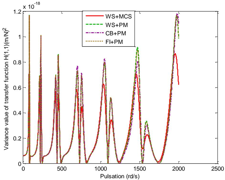
**Figure 3.** Variance value of transfer function  $H(1,1)$ , Monte Carlo Simulation (MCS) with 500 samples, Perturbation Method (PM) with Whole Structure (WS) and with Craig Bampton (CB) and Free Interface (FI) methods.  $\sigma_r = 2\%$ .
