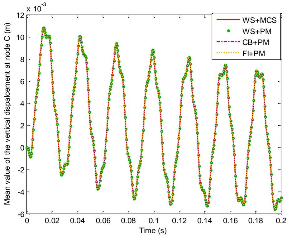
**Figure 4.** Mean value of the vertical displacement at the node C, Monte Carlo Simulation (MCS) with 500 samples, Perturbation Method (PM) with Whole Structure (WS) and with Craig Bampton (CB) and Free Interface (FI) methods.  $\sigma_r = 2\%$  .
