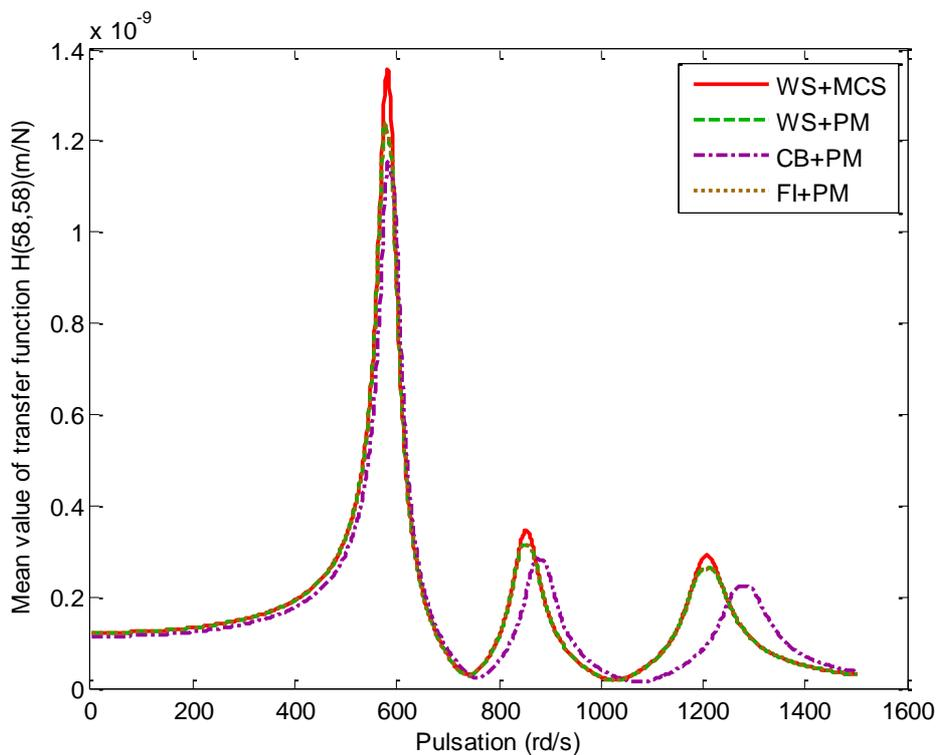
**Figure 8.** Mean value of transfer function  $H(58,58)$ , Monte Carlo Simulation (MCS) with 500 samples, Perturbation Method (PM) with Whole Structure (WS) and with Craig Bampton (CB) and Free Interface (FI) methods for  $\sigma_E = 2\%$ .
