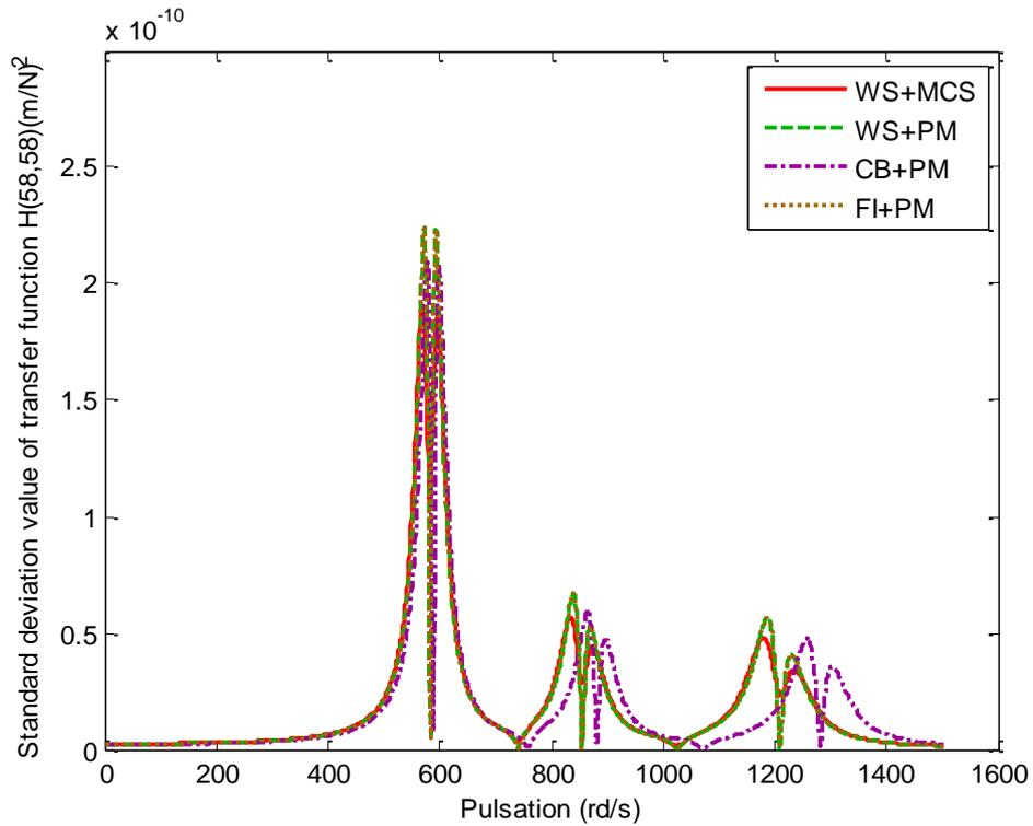
**Figure 9.** Standard deviation of transfer function  $H(58,58)$ , Monte Carlo Simulation (MCS) with 500 samples, Perturbation Method (PM) with Whole Structure(WS) and with Craig Bampton(CB) and Free Interface (FI) methods for  $\sigma_E = 2\%$  .
