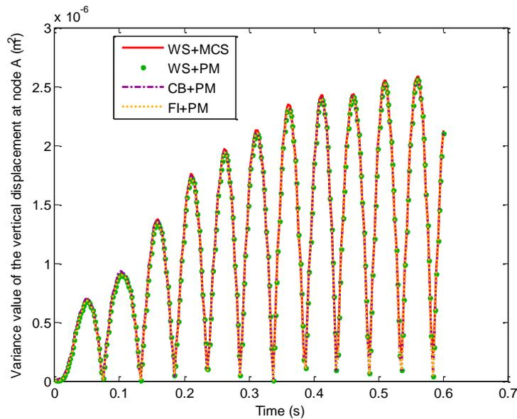
**Figure 11.** Variance value of the vertical displacement at the node A, Monte Carlo Simulation (MCS) with 500 samples, Perturbation Method (PM) with Whole Structure(WS) and with Craig Bampton(CB) and Free Interface (FI) methods for  $\sigma_E = 2\%$  .
