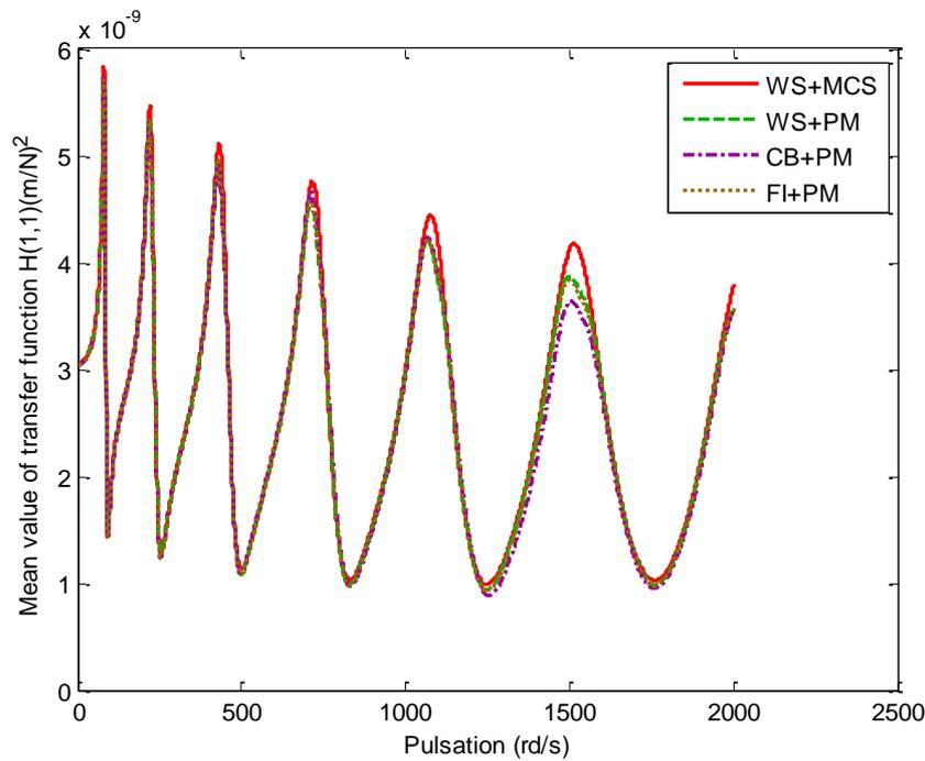
**Figure 2.** Mean value of transfer function  $H(1,1)$ , Monte Carlo Simulation (MCS) with 500 samples, Perturbation Method (PM) with Whole Structure (WS) and with Craig Bampton (CB) and Free Interface (FI) methods.  $\sigma_r = 2\%$ .
