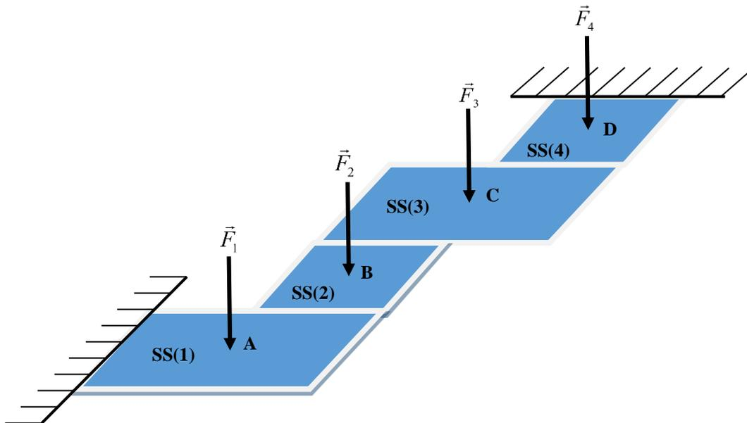
**Figure 6.** Example of discretisation of structure decomposed in substructures.
