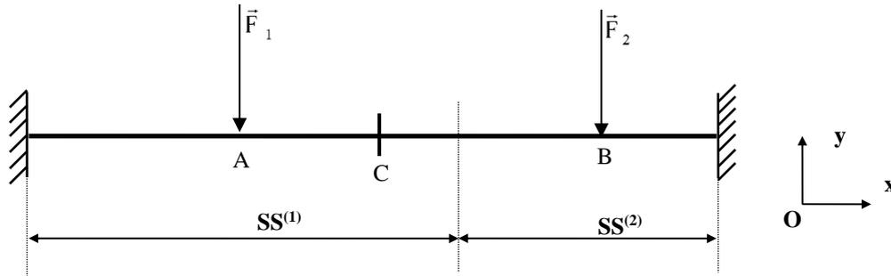
Figure 1. Sub structured clamped beam.
