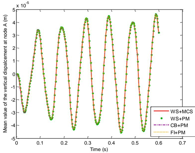
**Figure 10.** Mean value of the vertical displacement at the node A, Monte Carlo Simulation (MCS) with 500 samples, Perturbation Method (PM) with Whole Structure(WS) and with Craig Bampton(CB) and Free Interface (FI) methods for  $\sigma_E = 2\%$  .
