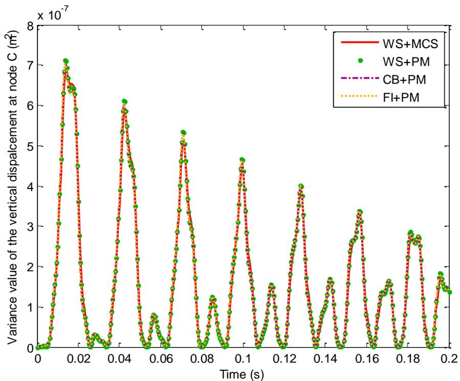
**Figure 5.** Variance value of the vertical displacement at the node C, Monte Carlo Simulation (MCS) with 500 samples, Perturbation Method (PM) with Whole Structure (WS) and with Craig Bampton (CB) and Free Interface (FI) methods.  $\sigma_r = 2\%$  .
