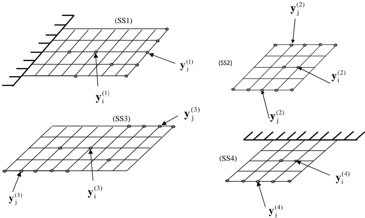
**Figure 7.** Four substructures (SS1, (SS2), (SS3) and (SS4), interface dof vector  $\mathbf{y}_j^{(k)}$  and internal dof vector  $\mathbf{y}_i^{(k)}$
