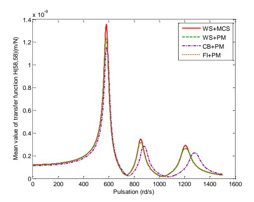
Figure 8. Mean value of transfer function H(58,58), Monte Carlo Simulation (MCS) with 500 samples, Perturbation Method(PM) with Whole Structure(WS) and with Craig Bampton(CB) and Free Interface (FI) methods for  $\sigma_E = 2\%$ .
