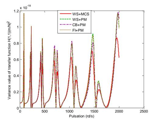
**Figure 3.** Variance value of transfer function H(1,1), Monte Carlo Simulation (MCS) with 500 samples, Perturbation Method (PM) with Whole Structure (WS) and with Craig Bampton (CB) and Free Interface (FI) methods.  $\sigma_r = 2\%$ .
