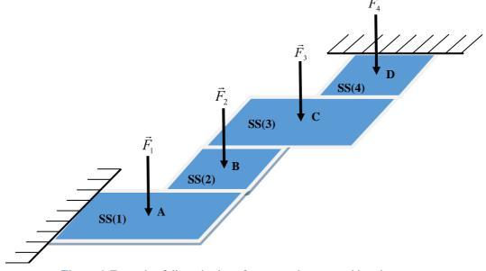
Figure 6. Example of discretisation of structure decomposed in substructures.
