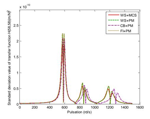
Figure 9. Standard deviation of transfer function H(58,58), Monte Carlo Simulation (MCS) with 500 samples, Perturbation Method (PM) with Whole Structure(WS) and with Craig Bampton(CB) and Free Interface (FI) methods for  $\sigma_E = 2\%$ .
