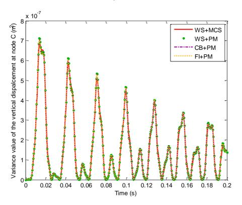
Figure 5. Variance value of the vertical displacement at the node C, Monte Carlo Simulation (MCS) with 500 samples, Perturbation Method (PM) with Whole Structure (WS) and with Craig Bampton (CB) and Free Interface (FI) methods.  $\sigma_r = 2\%$ .
