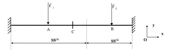
Figure 1. Sub structured clamped beam.
