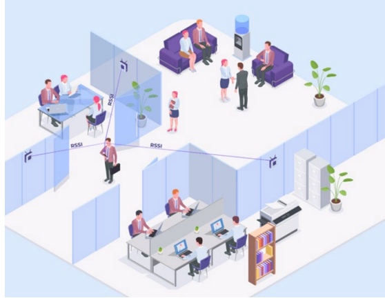
Figure 9. Schematic diagram of Wi-Fi-based IPS principle
