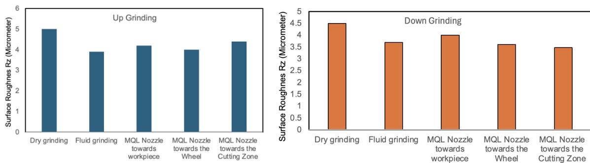
Figure 7. Effect of nozzle orientation on surface roughness [101]
