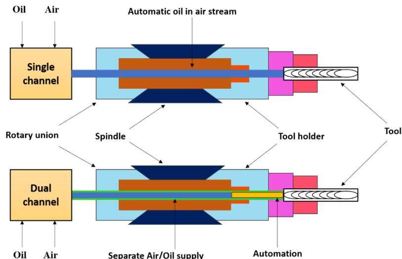
Figure 2. Internal delivery system of MQL technology
