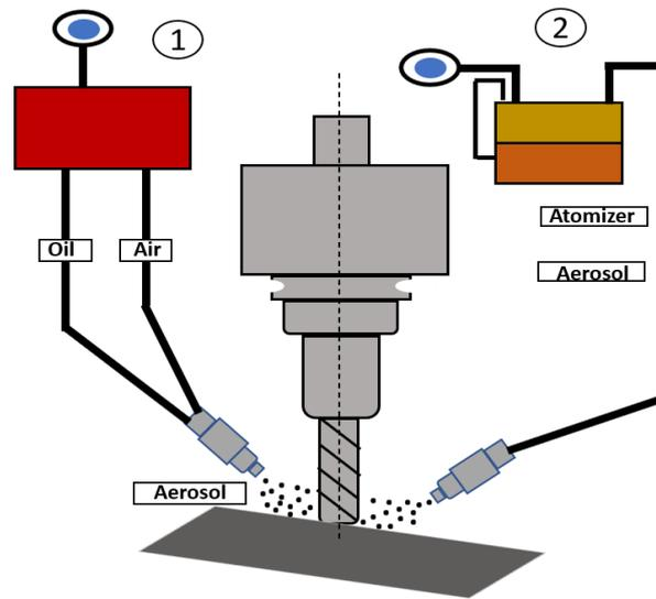
Figure 3. External delivery system of MQL technology: 1. Ejector nozzle, 2. Conventional [28]
