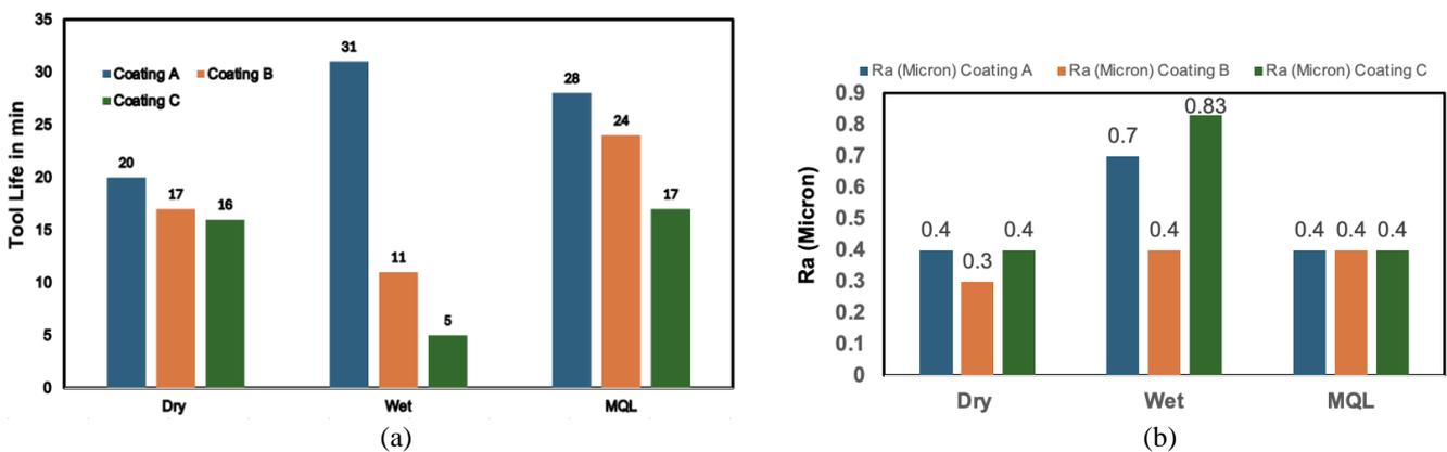
Figure 4. (a) Tool life and (b) surface finish for three types of machining conditions: dry, wet, and MQL [34]
