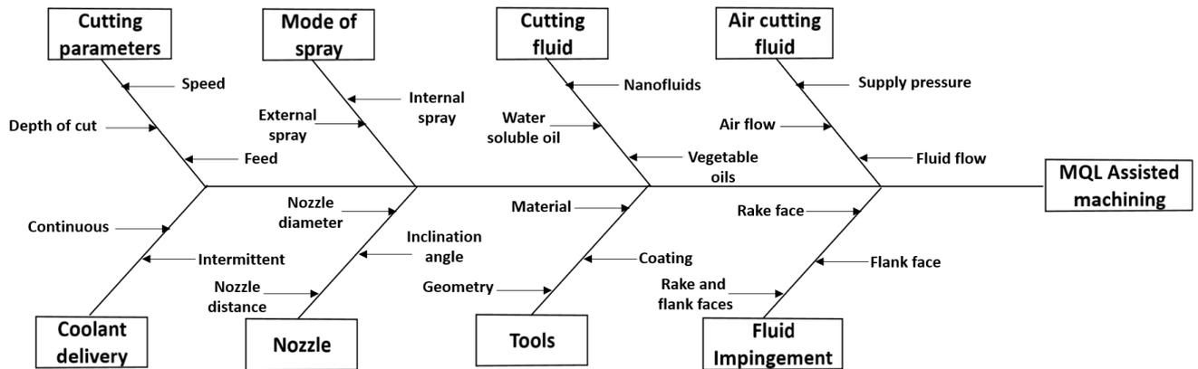
Figure 6. Fishbone like structure displaying MQL assisted machining parameters and conditions [35]
