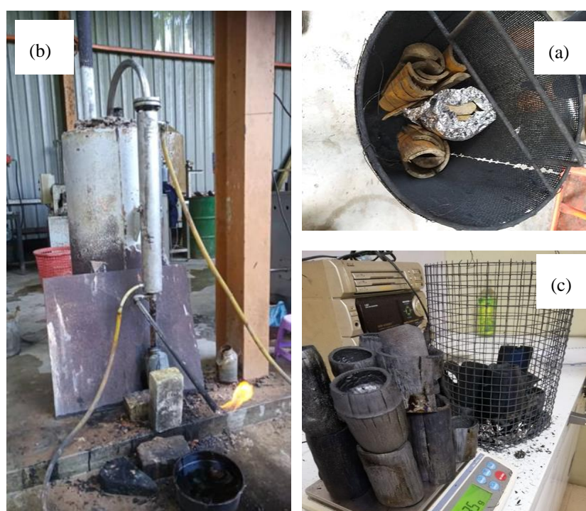
Figure 1. Process of bamboo charcoal production using pyrolyser (a) Bamboo loaded into pyrolyser basket; (b) Pyrolysis using pyrolyser; (c) Bamboo charcoal.
